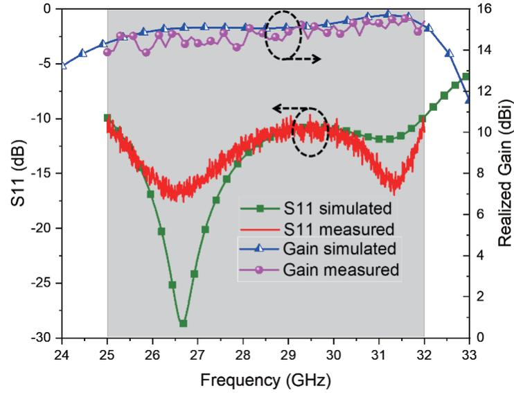
Figure 8. Return loss and realized gain of the proposed antenna array.
