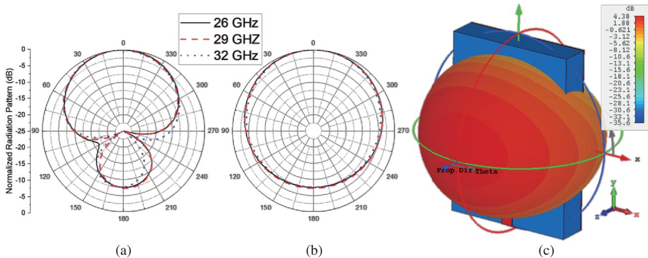
Figure 3. Radiation patterns of the proposed antenna element (a)  $E$ -plane (b)  $H$ -plane (c) 3D.
