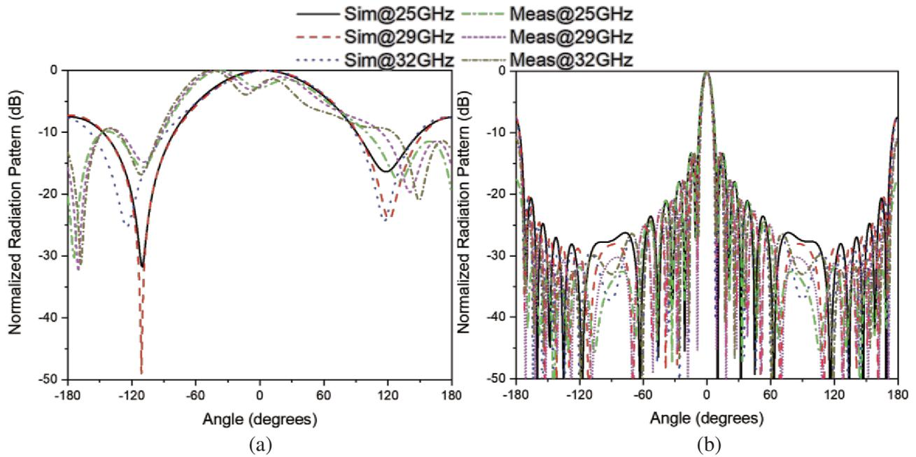
Figure 9. Simulated and measured radiation patterns of the proposed antenna array (a) *E*-plane (b) *H*-plane.
