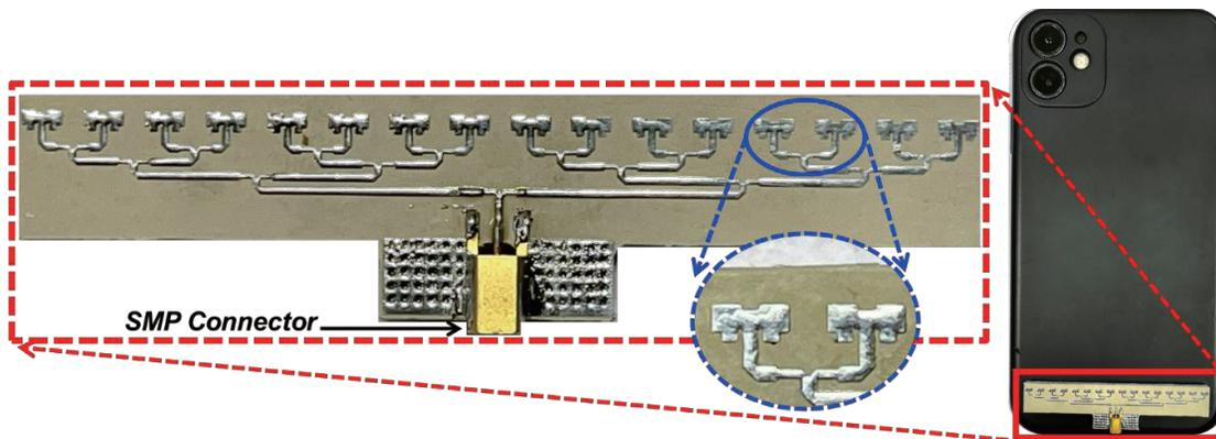
**Figure 7.** Prototype of the proposed antenna array.
