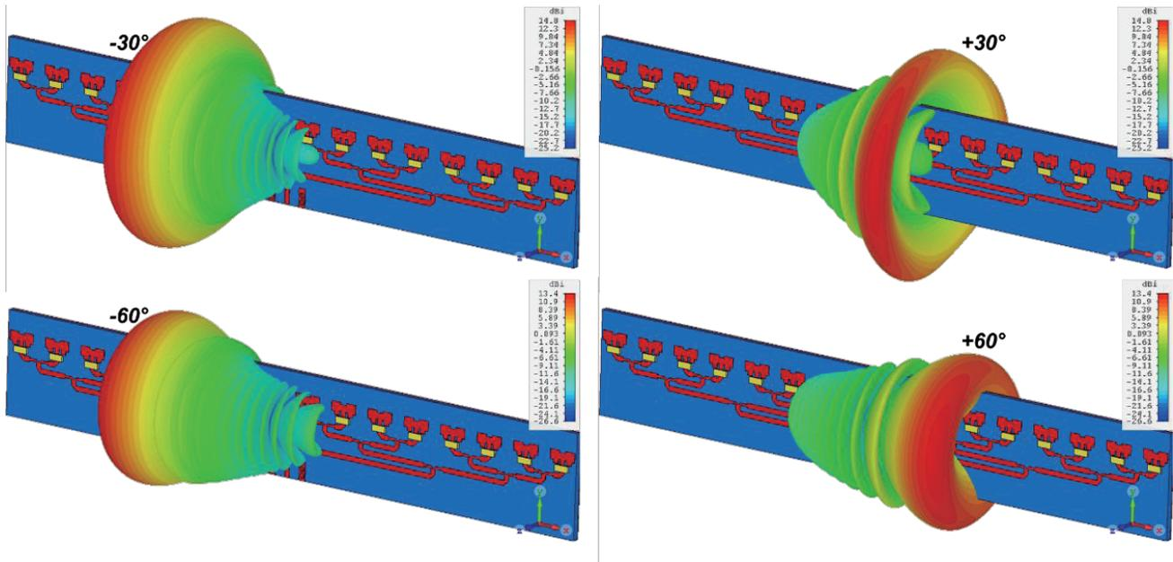
Figure 11. The radiation patterns of the proposed antenna array at different steering angles.
