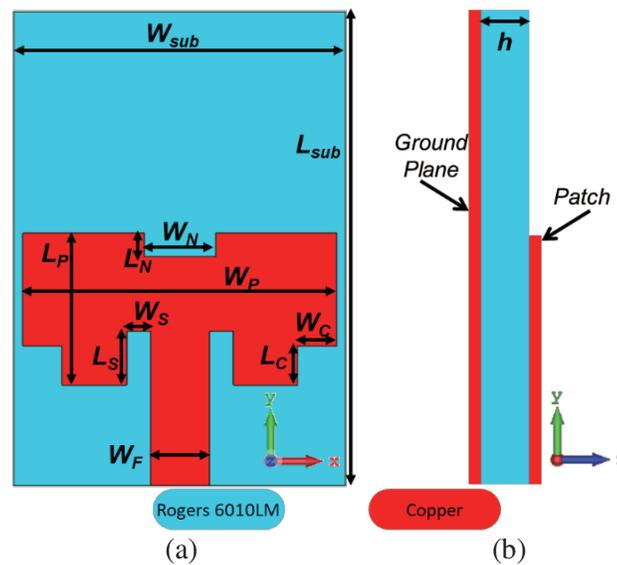
**Figure 1.** The proposed antenna element (a) front view (b) side view.
