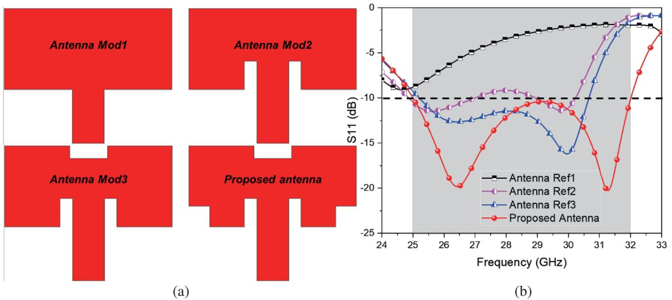
Figure 2. Model and proposed antennas (a) evolution (b) return loss.
