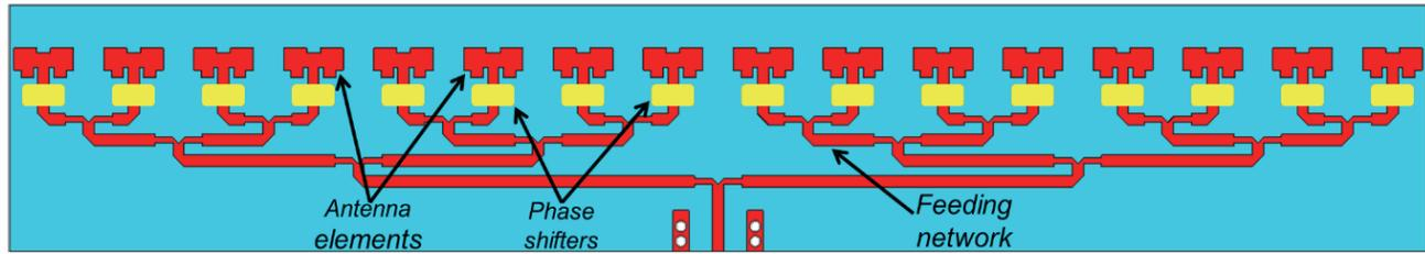
Figure 10. The proposed antenna array with digital phase shifters.
