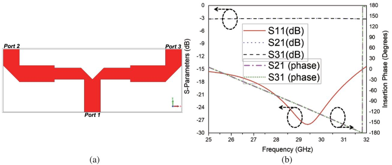
Figure 5. An example of the T-dividers in the feeding network (a) structure (b)  $S$ -parameters.
