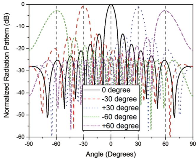
**Figure 12.** The normalized radiation patterns of the proposed antenna array at *H*-plane at different steering angles.
