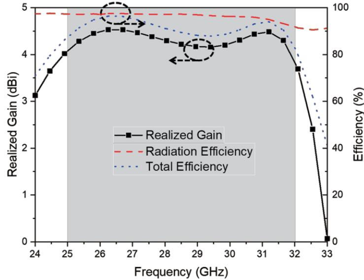
Figure 4. Realized gain and efficiencies of the antenna element.
