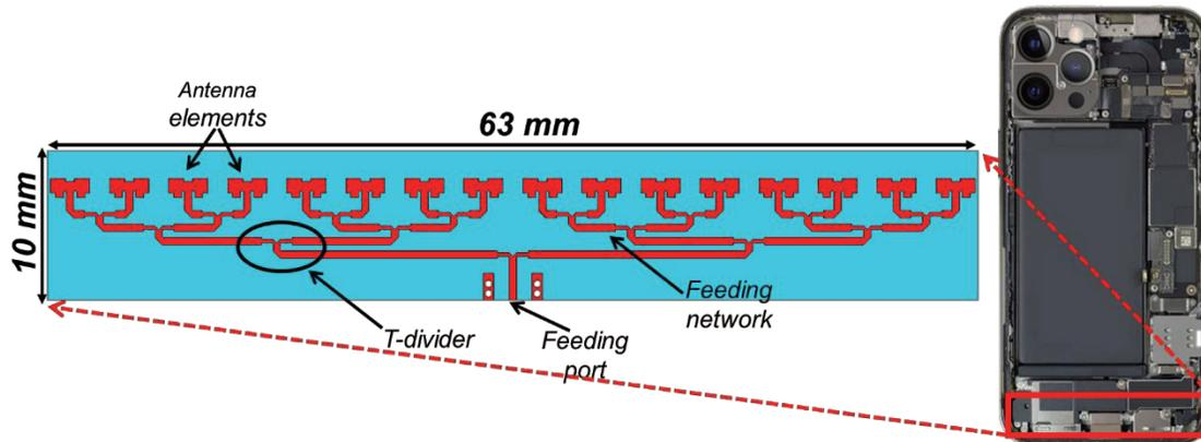
**Figure 6.** Structure of the proposed antenna array.
