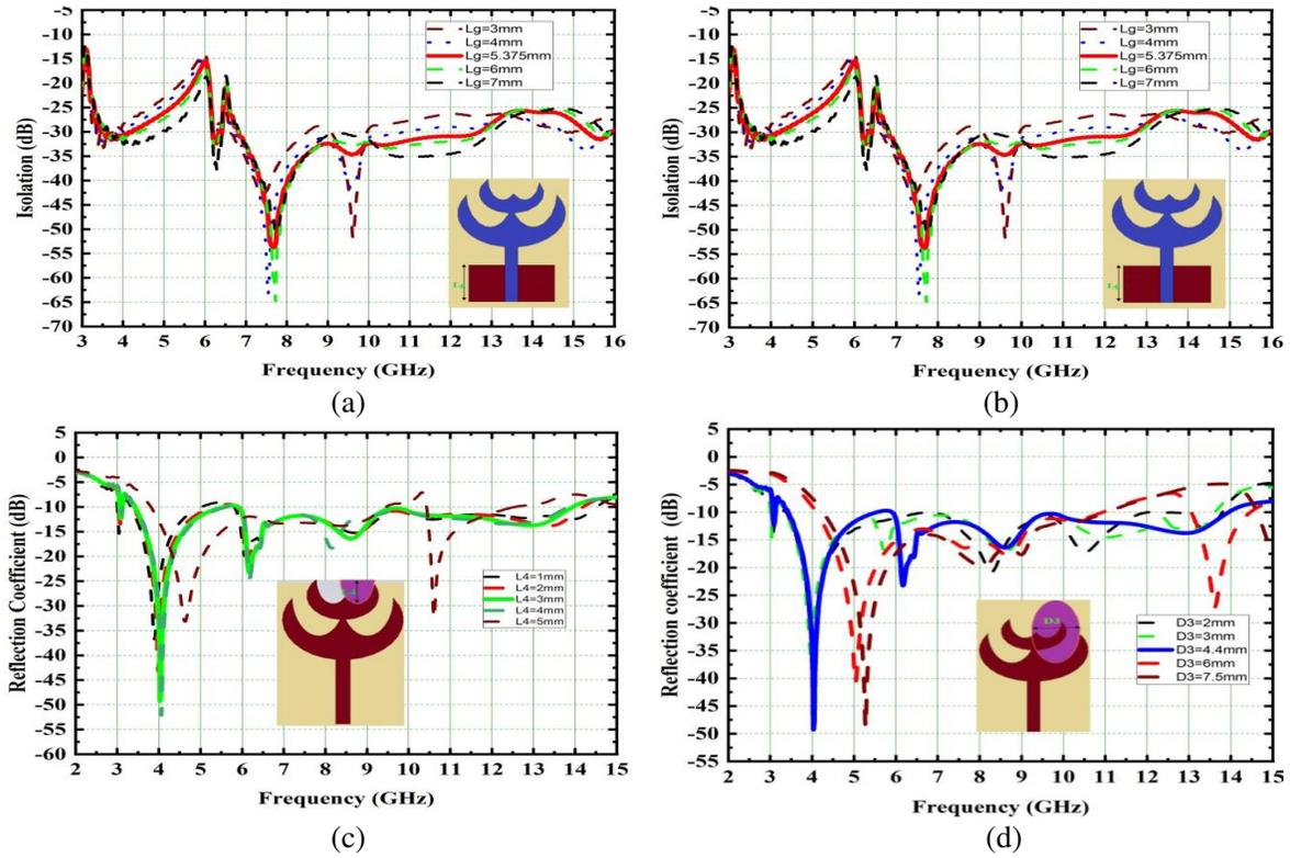
**Figure 2.** Parametric variations of single flower radiator w.r.t.. (a) Length of the ground  $L_g$ . (b) Isolation due to  $L_g$ . (c) Variations in  $L_4$  (height of the Upper Petal). (d) Variations in  $D_3$  (Diameter of the lower petal).
