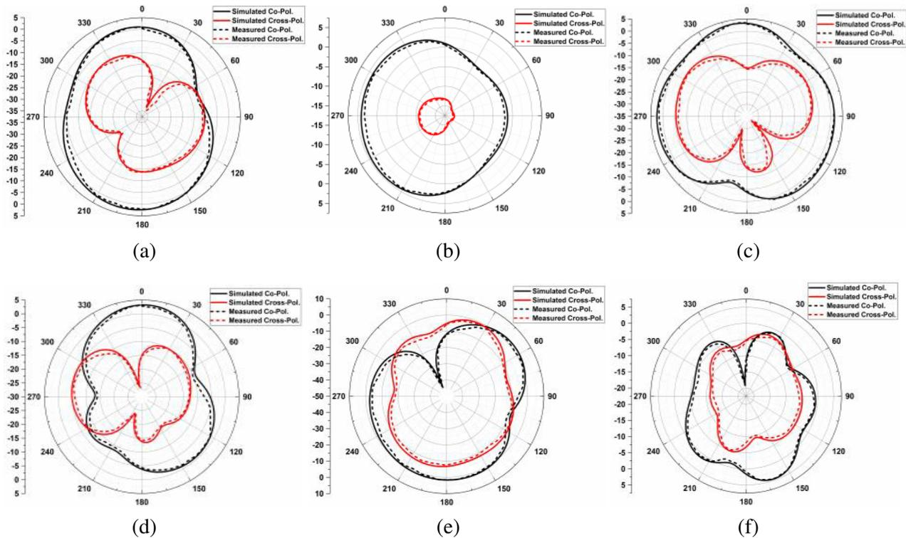
**Figure 14.** The flower shaped  $4 \times 4$  antenna radiation pattern of  $E$ -Plane at (a) 4.1 GHz, (c) 6.2 GHz, (e) 8.6 GHz and  $H$ -plane at (b) 4.1 GHz, (d) 6.2 GHz, (f) 8.6 GHz.
