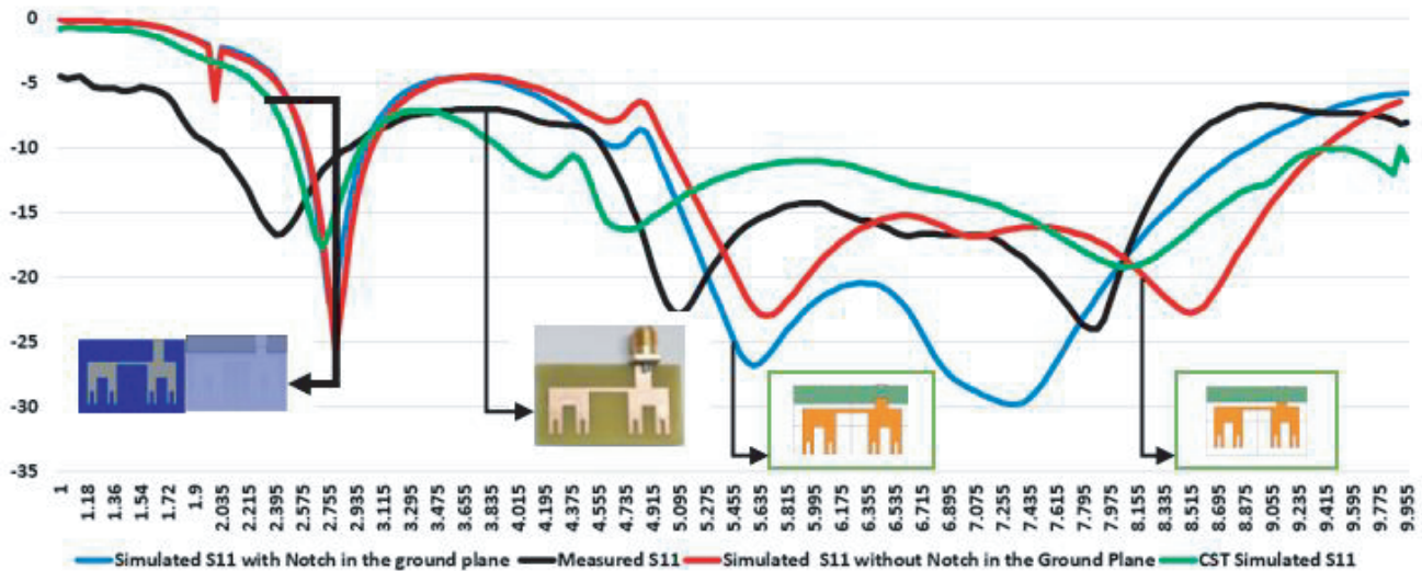
Figure 17. S_{11} comparison of Mentor graphics simulation, CST simulation and Measured results.
