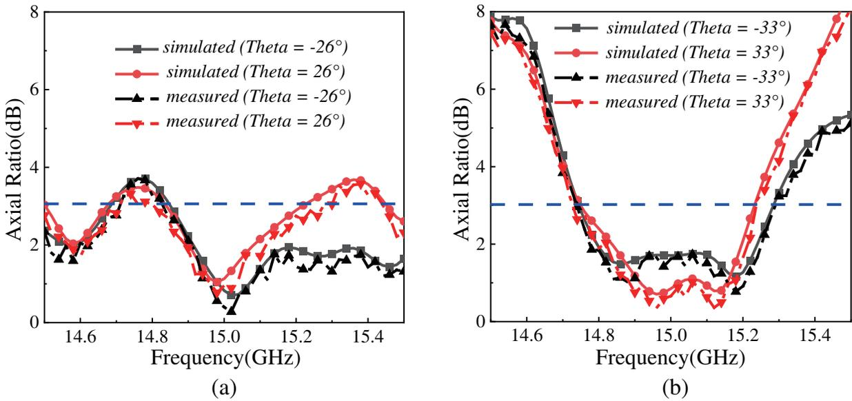
**Figure 13.** Axial ratio when different circularly polarized waves are incident (a) right-handed circularly polarized wave,  $\Phi = 90^\circ$  (b) left-handed circularly polarized wave,  $\Phi = 0^\circ$ .
