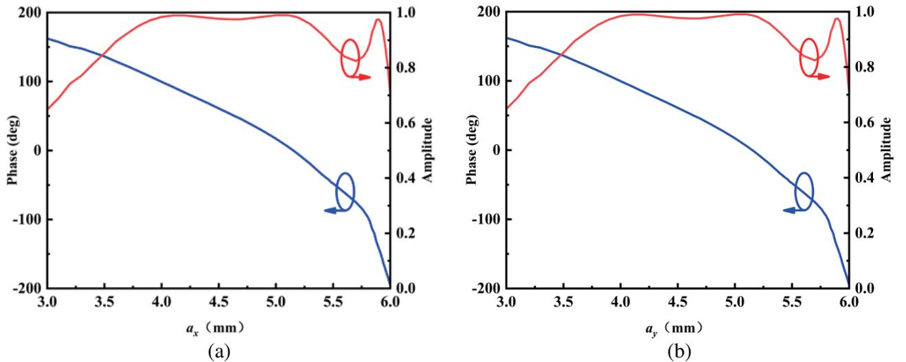
**Figure 2.** The transmission phase and amplitude of the unit cell (a) changed with  $a_x$  when the incident wave is  $x$ -polarization, (b) changed with  $a_y$  when the incident wave is  $y$ -polarization.
