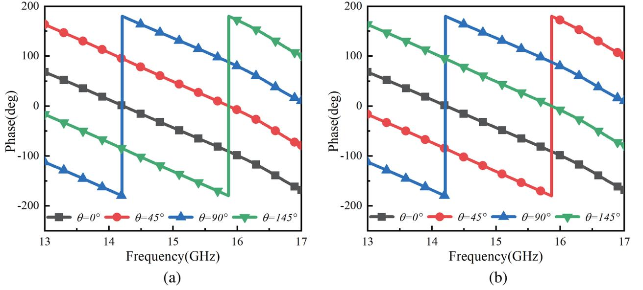
**Figure 6.** The phase response of the unit cell by rotating  $\theta$  when electromagnetic waves are incident in different polarization directions (a) left-handed circular polarization (b) right-handed circular polarization.
