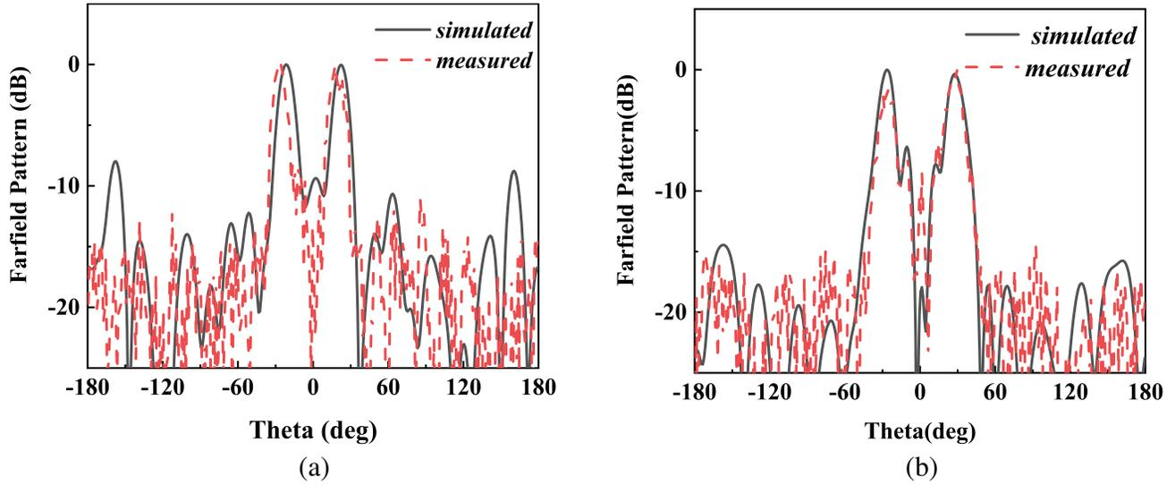
**Figure 12.** Cartesian pattern of different circularly polarized incident waves (a) right-handed circularly polarized wave,  $\Phi = 90^\circ$  (b) left-handed circularly polarized wave,  $\Phi = 0^\circ$ .
