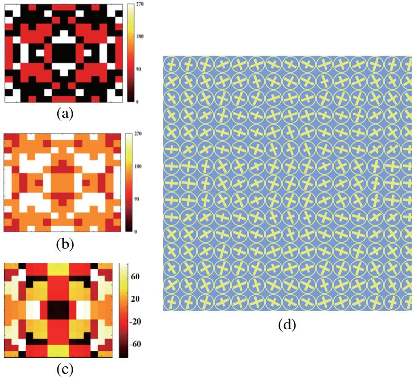
**Figure 9.** Schematic diagram of phase distribution and array model (a)  $x$ -polarization phase distribution (b)  $y$ -polarization phase distribution (c) rotation angle distribution (d) array model.
