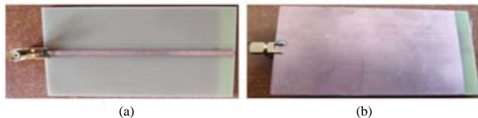
Figure 7. (a) Front view of array without DRA. (b) Back view of an array without DRA.
