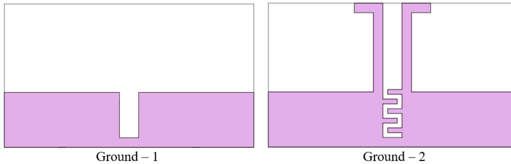
Figure 6. Evolution stages of the ground plane of proposed MIMO antenna.
