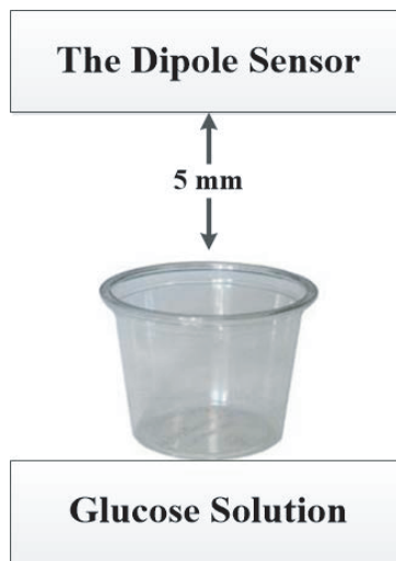
Figure 3. The Dipole Sensor and its proximity to the solution.
