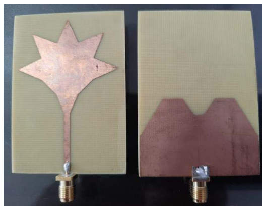
Figure 9. Fabricated antenna hardware front view (patch) and back view (ground).
