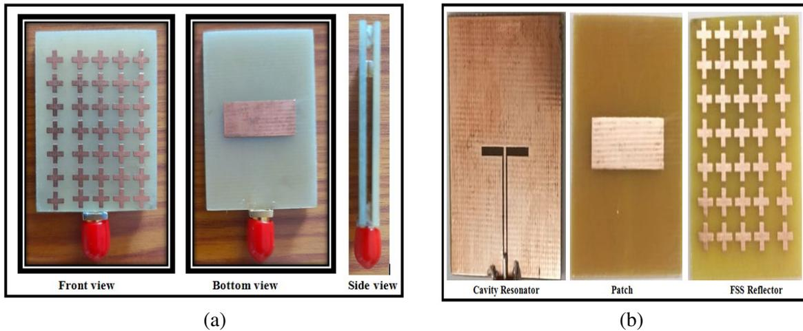
Figure 4. A prototype of the proposed antenna: Front view, bottom view and side view.
