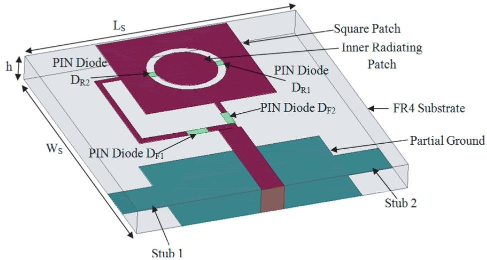
Figure 4. Antenna design with PIN diodes.
