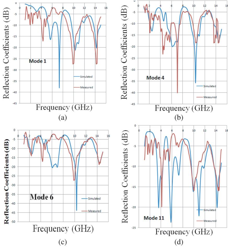
**Figure 8.** Measured and simulated reflection coefficients of antenna in (a) mode 1, (b) mode 4, (c) mode 6 and (d) mode 11.
