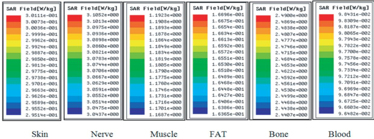
Figure 14. SAR values on six tissues of human arm with antenna in mode ‘15’ at 2.624 GHz.
