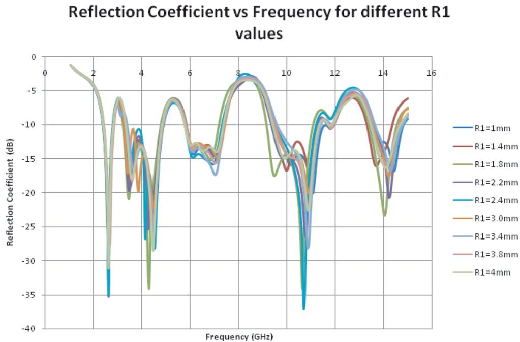
Figure 5. Inner radiating patch radius parametric analysis.
