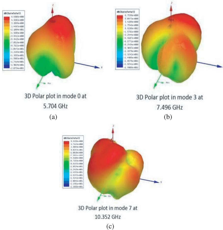
Figure 10. 3D Polar plots of antenna in (a) mode 0 at 5.704 GHz, (b) in mode 3 at 7.496 GHz and (c) mode 7 at 10.352 GHz.
