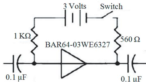
Figure 3. PIN diode switch.
