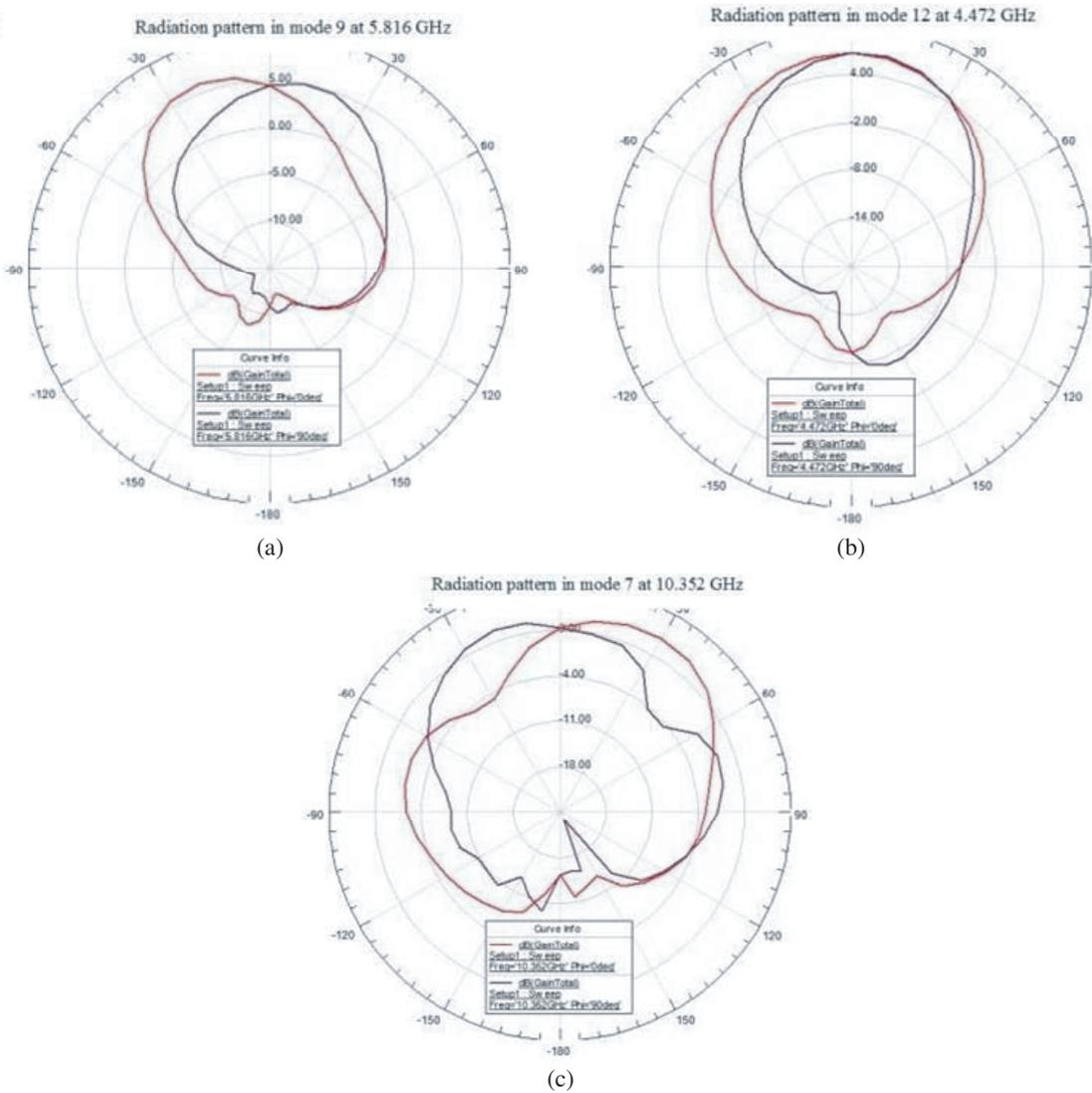
**Figure 11.** Radiation patterns of antenna in (a) mode 9 at 5.816 GHz, (b) in mode 12 at 4.472 GHz and (c) mode 7 at 10.352 GHz.
