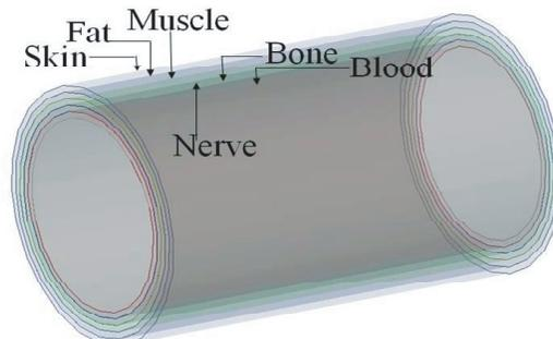
**Figure 12.** Six layer human arm model in HFSS.
