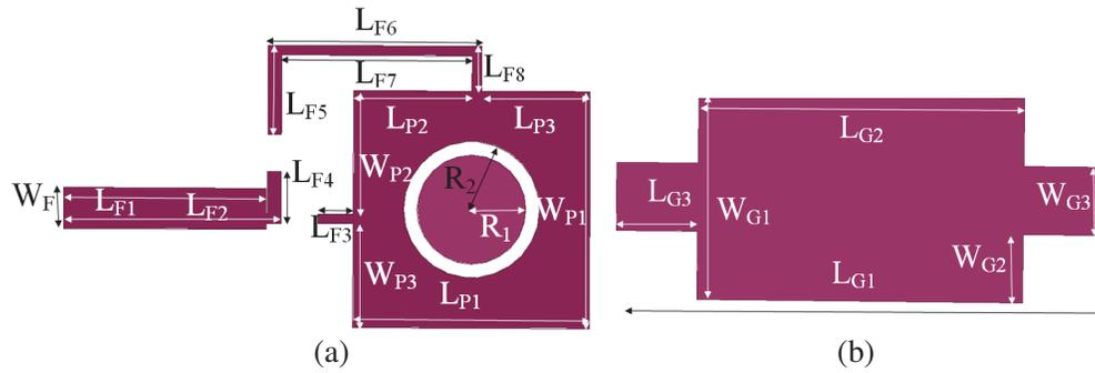
Figure 1. (a) Antenna patch. (b) Antenna ground.
