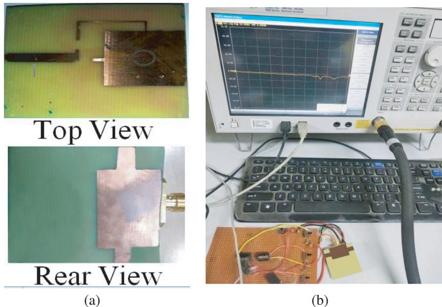
**Figure 6.** (a) Fabricated antenna. (b) Measurement set up with VNA.
