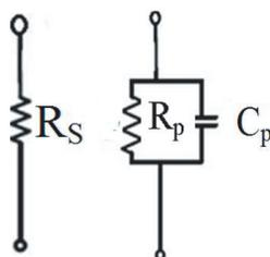
Figure 2. Equivalent Circuit of PIN diode.
