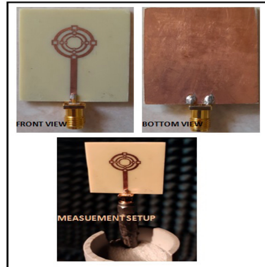
Figure 4. Photograph of prototype (front and bottom view) and measurement setup.
