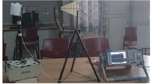
Figure 10. Experimental set up for radiation pattern measurement of antenna with EBG.
