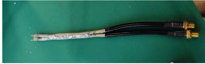
Figure 10. Semi-rigid differential probe test fixture for impedance measurement.
