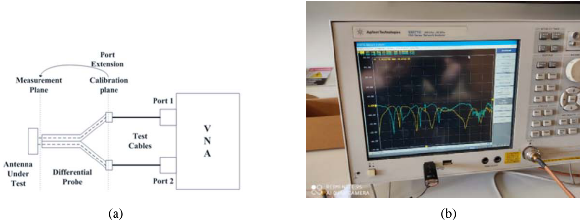
Figure 11. (a) Layout configuration of measurement setup with differential probe, (b) impedance measurement setup with VNA.
