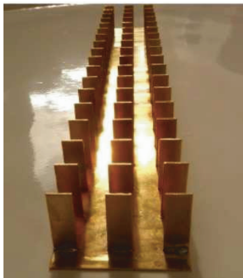
Figure 7. Lighter metamaterial structure designed at 1.1 GHz.
