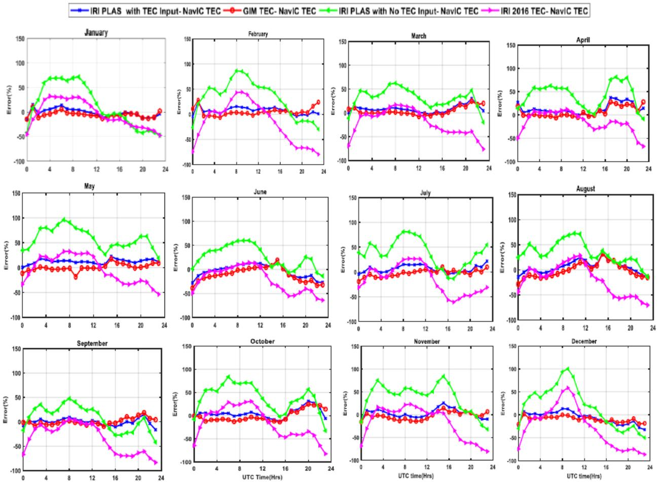
**Figure 6.** Error percentages of estimated VTEC by standard models (IRI Plas with TEC input, GIM, IRI Plas with no TEC input and IRI-2016) from NavIC TEC for geomagnetic disturbed days during the year 2017.
