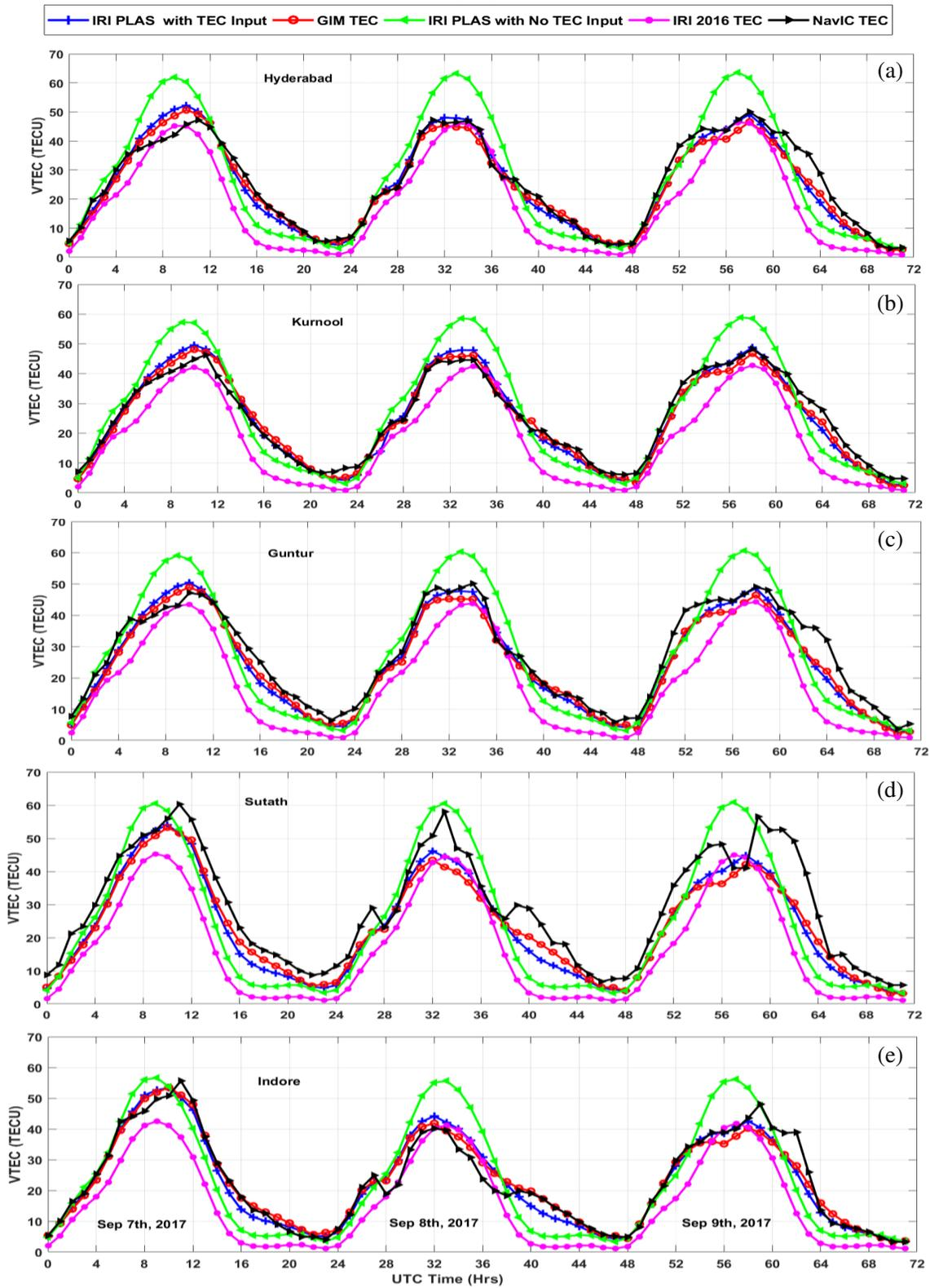
**Figure 17.** Variation of VTEC due to models and NavIC on geomagnetic storm during September 7th to 9th, 2017 over (a) Hyderabad, (b) Kurnool, (c) Gunture, (d) Surath, (e) Indore stations.
