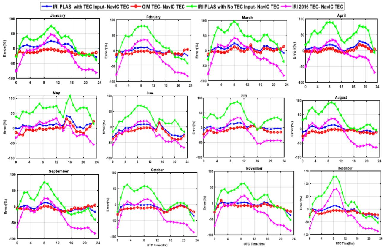
**Figure 4.** Error percentages of estimated VTEC by standard models (IRI Plas with TEC input, GIM, IRI Plas with no TEC input and IRI-2016) from NavIC TEC for geomagnetic quiet days during the year 2017.
