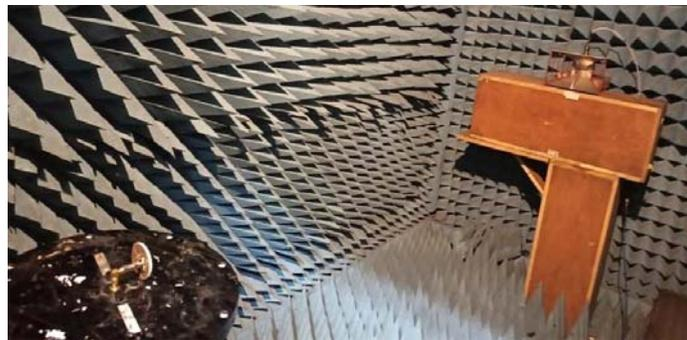
**Figure 10.** Projected antenna in an anechoic chamber.
