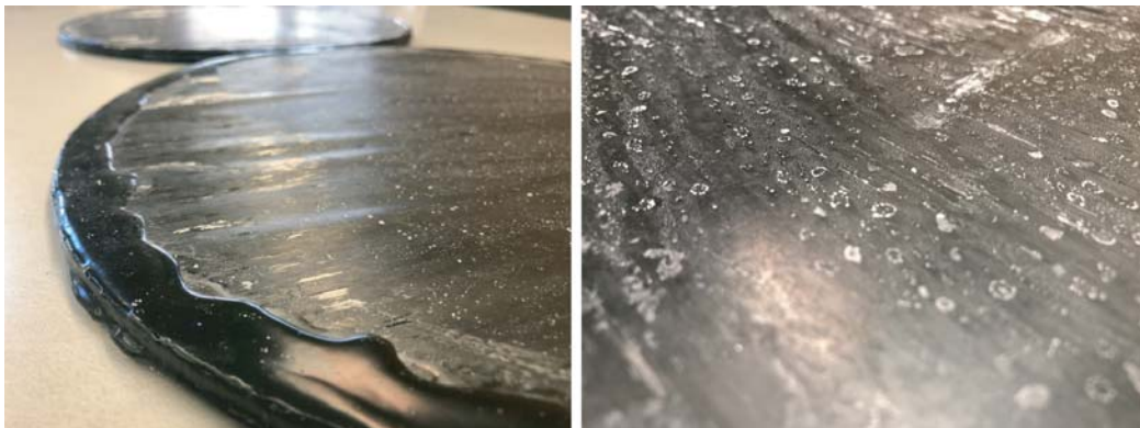
Figure 1. Rippling and salt crystal formation due to a fiber-matrix weakening seen after salt water exposure and removed from the chamber after five days.
