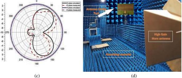
Figure 15. E plane and H plane (measured vs simulated) at the various resonating frequency and measurement setup. (a) 1.83 GHz, (b) 3.65 GHz, (c) 5.59 GHz, (d) chamber set up.
