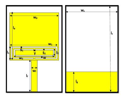
Figure 2. Geometry of CSRR engraved rectangular antenna and its parameters.
