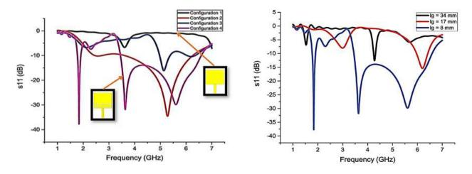
Figure 3.  $S_{11}$  comparison (Configuration 1 to 4). Figure 4. Ground length analysis.
