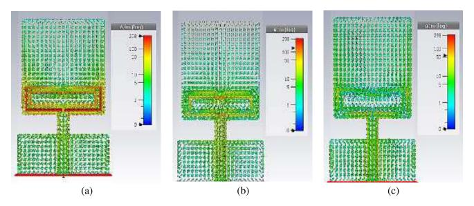
Figure 14. Surface current distribution at the various resonating frequency. (a) 1.83 GHz, (b) 3.65 GHz, (c) 5.59 GHz.
