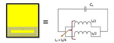
Figure 9. Equivalent circuit of CSRR.
