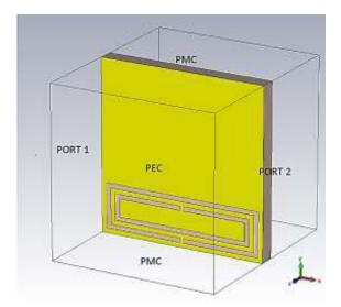
Figure 10. S parameter extraction set up.
