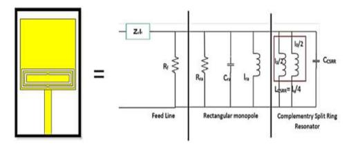
Figure 13. Equivalent circuit of the proposed antenna.
