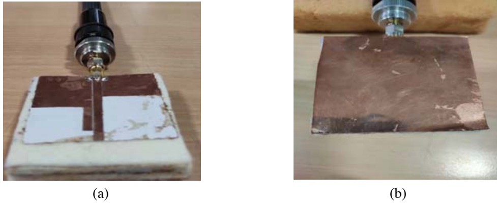
Figure 12. Fabricated antenna, (a) front view, (b) back view.
