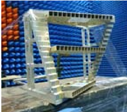
Figure 8. Photograph of measurement setup and the fabricated subarrays.
