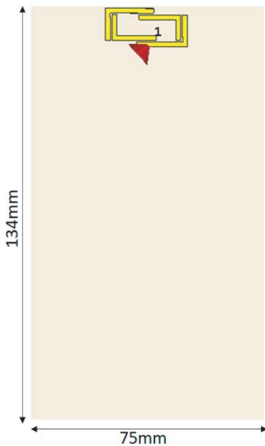
Figure 2. The Complete geometry of the folded dipole on a substrate of a size of a mobile phone.
