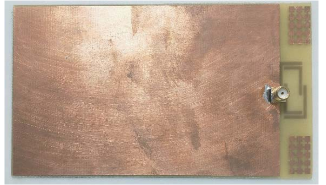
Figure 20. Fabricated folded dipole antenna with a partial ground plane loaded by printed DGS.
