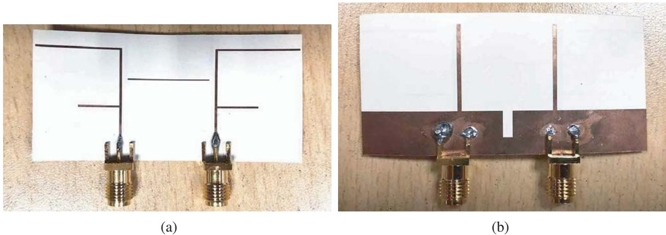
**Figure 5.** Fabricated antenna. (a) Front. (b) Back.
