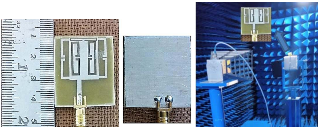
Figure 15. Top and bottom view of the fabricated antenna & measurement setup.
