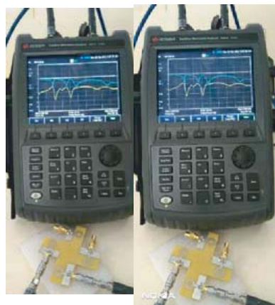
Figure 16. Four element MIMO antenna prototype with VNA measurement setup.
