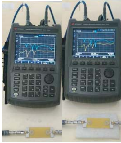
Figure 10. Two element MIMO antenna prototype with VNA measurement setup.
