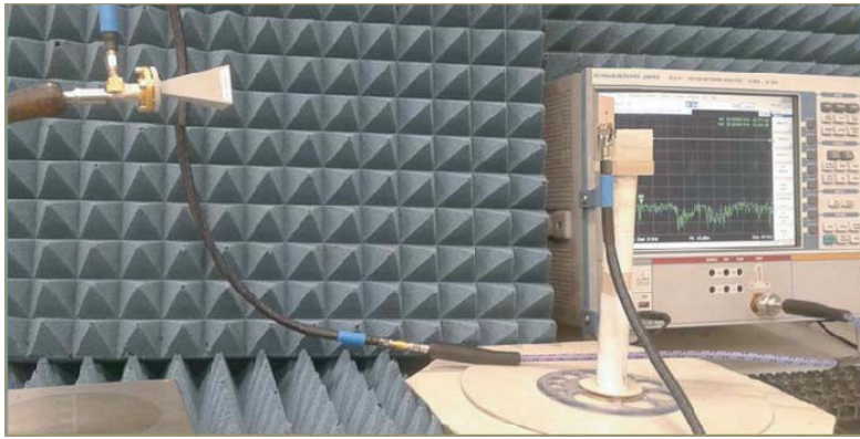
Figure 12. Experimental setup for measuring the radiation pattern and gain of the quad-band antenna.
