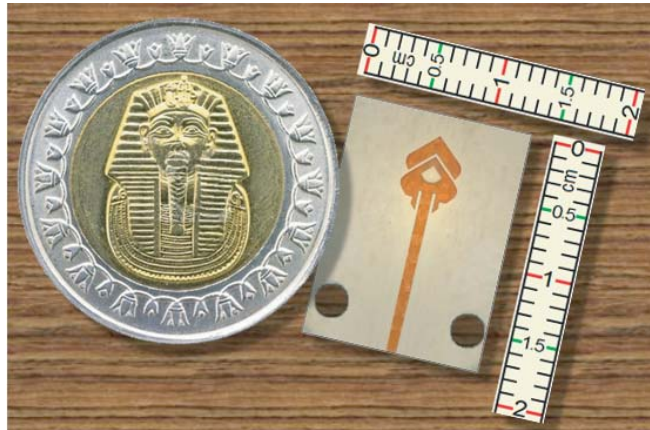
Figure 9. Fabricated prototype of the proposed quad-band patch antenna with its size compared to a metal coin of standard size.
