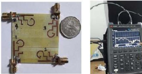
**Figure 8.** Testing of prototype using Keysight fieldfox microwave Analyzer N9918A.
