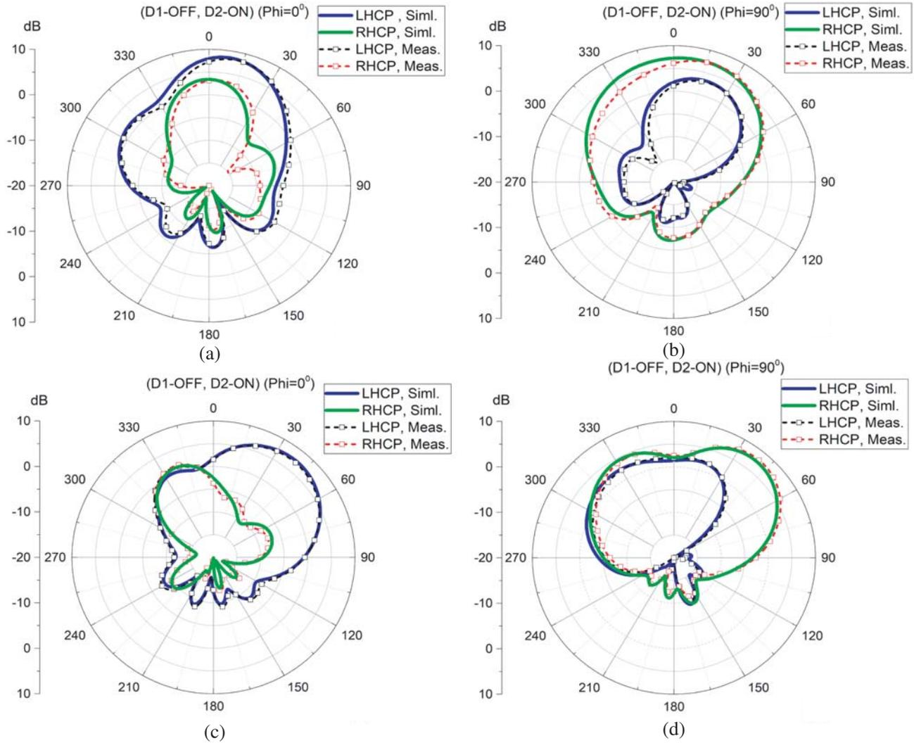
**Figure 11.** Simulated and Measured radiation patterns for D1-OFF, D2-ON state at (a) 6.2 GHz ( $\phi = 0^\circ$ ), (b) 6.2 GHz ( $\phi = 90^\circ$ ), (c) 9.3 GHz ( $\phi = 0^\circ$ ), (d) 9.3 GHz ( $\phi = 90^\circ$ ).
