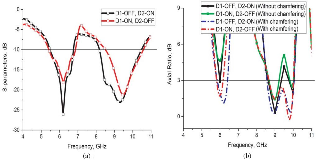
**Figure 6.** (a) Simulated *S*-parameters, dB. (b) Axial ratio, dB (with and without chamfering).
