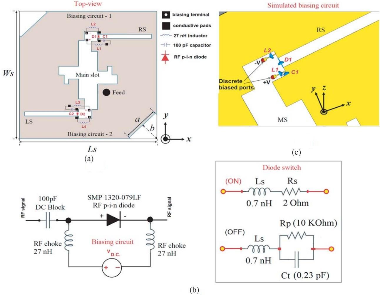
**Figure 3.** (a) Top view of antenna circuit. (b) Biasing circuit configuration and switching mechanism. (c) Simulated biasing circuit.
