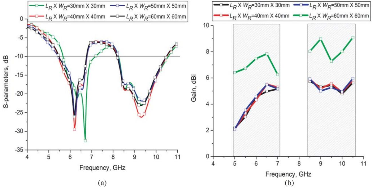
**Figure 8.** Effects of (a)  $S$ -parameters, dB, (b) Gain, dBi in reflector size  $L_R \times W_R$  variation.
