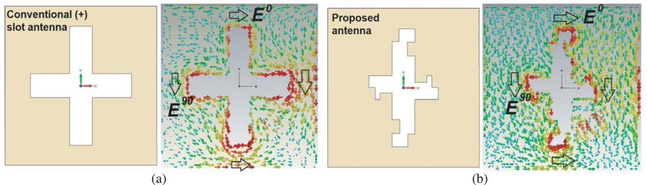
**Figure 1.** Current distributions in (a) Conventional (+) slot antenna, (b) Proposed slot antenna.
