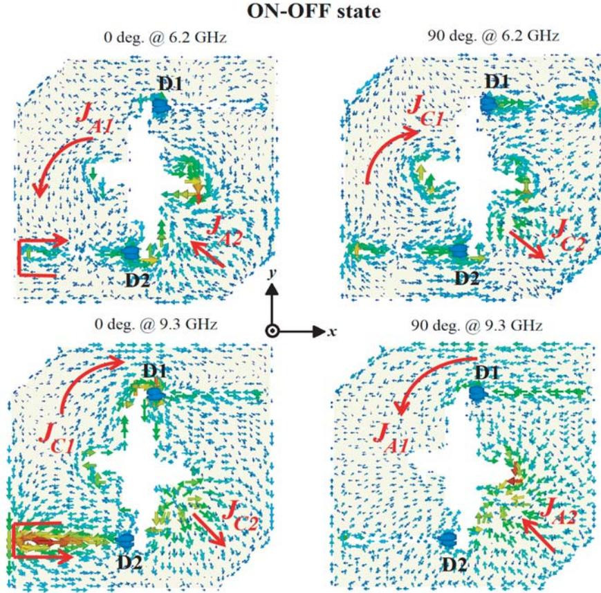
**Figure 5.** Surface current streamlines at 6.2 GHz and 9.3 GHz for D1-ON, D2-OFF state.
