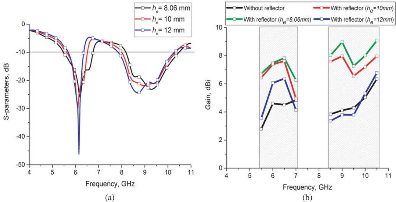
**Figure 7.** Effects of (a)  $S$ -parameters, dB, (b) Gain, dBi in reflector height  $h_e$  variation.
