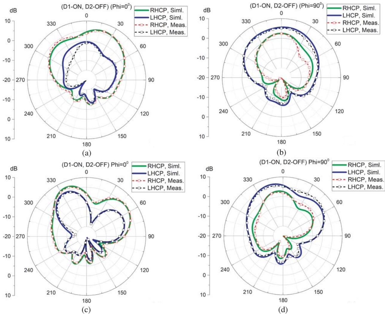
**Figure 12.** Simulated and Measured radiation patterns for D1-ON, D2-OFF state at (a) 6.2 GHz ( $\phi = 0^\circ$ ), (b) 6.2 GHz ( $\phi = 90^\circ$ ), (c) 9.3 GHz ( $\phi = 0^\circ$ ), (d) 9.3 GHz ( $\phi = 90^\circ$ ).
