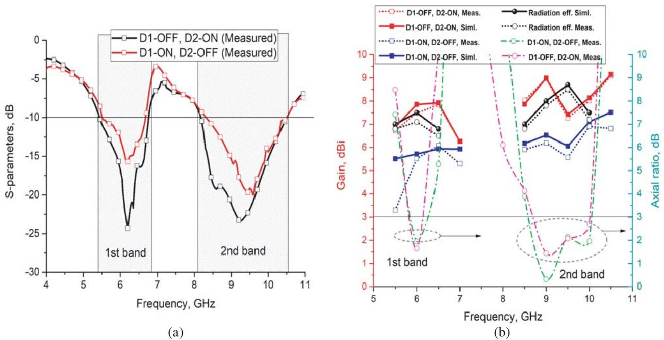
**Figure 10.** Validation: Measured (a)  $S$ -parameters, dB and (b) Gain, dBi with Axial ratio, dB & Radiation Efficiency, linear scale of proposed antenna.
