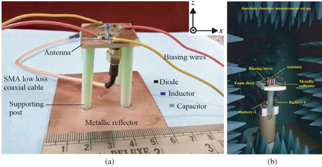
**Figure 13.** (a) Fabricated prototype. (b) Antenna measurement set-up in anechoic chamber.
