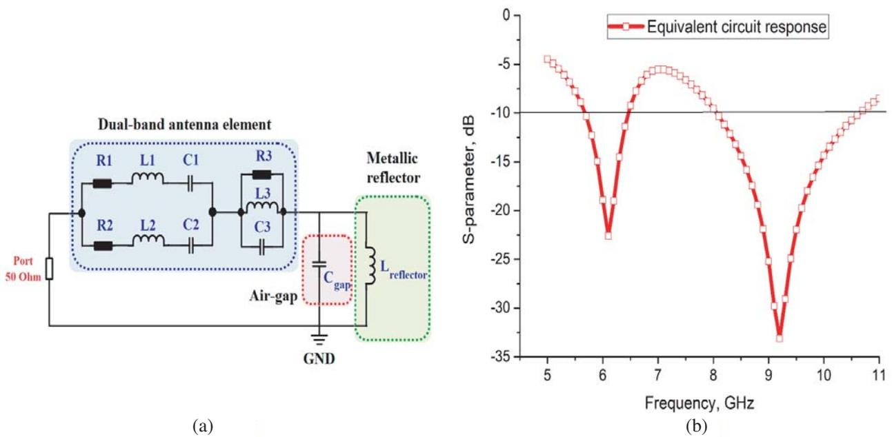
**Figure 9.** (a) Equivalent circuit of proposed antenna configuration. (b) Equivalent circuit response. ( $Z_0 = 50 \Omega$ ,  $R1 = 26.3 \Omega$ ,  $L1 = 7.608 \text{ nH}$ ,  $C1 = 0.0915 \text{ pF}$ ,  $R2 = 23.15 \Omega$ ,  $L2 = 2.318 \text{ nH}$ ,  $C2 = 0.133 \text{ pF}$ ,  $R3 = 30.5 \Omega$ ,  $L3 = 8.75 \text{ nH}$ ,  $C3 = 0.098 \text{ pF}$ ,  $L_{reflector} = 0.5 \text{ nH}$ ,  $C_{gap} = 10 \text{ pF}$ ).
