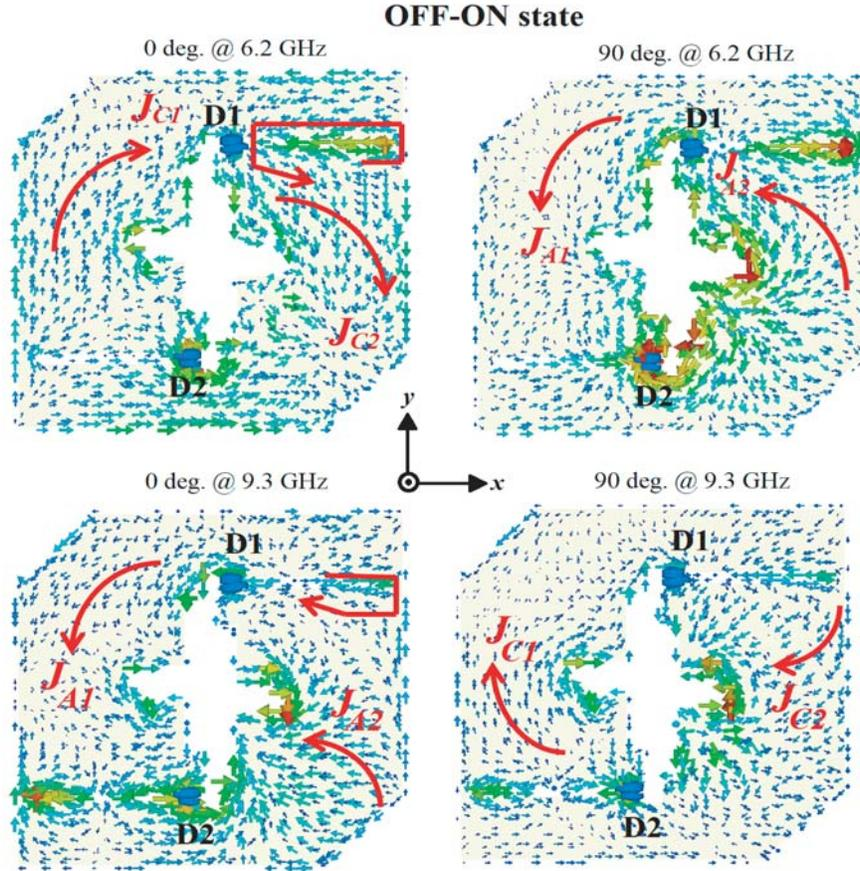
**Figure 4.** Surface current streamlines at 6.2 GHz and 9.3 GHz for D1-OFF, D2-ON state.
