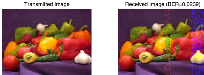
Figure 13. Transmitted and received image for 64-QAM rate 3/4 modulation techniques.
