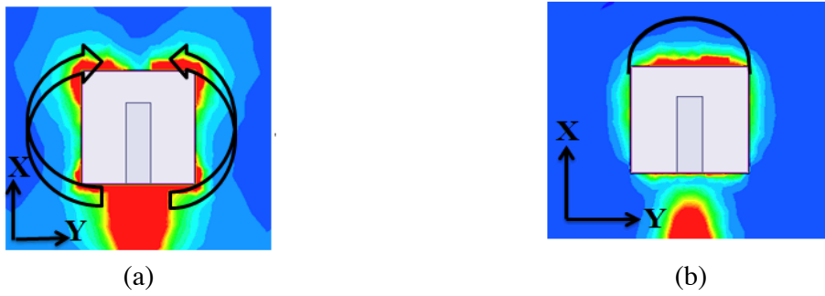
Figure 14. Field distribution over the aperture at 5.6 GHz. (a) E -field, (b) H -field.
