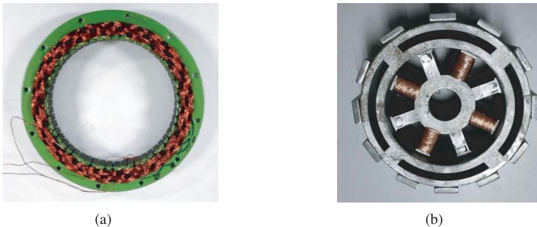
Figure 20. Prototype of PM motor and BHMB. (a) Stator of external PM motor. (b) Prototype of BHMB.
