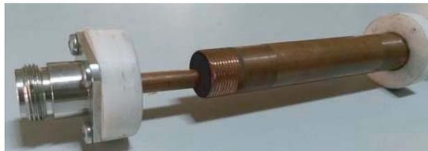
**Figure 2.** Design feature for varying dielectric.
