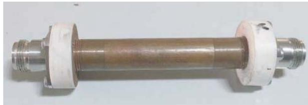
**Figure 1.** Coaxial transmission line.
