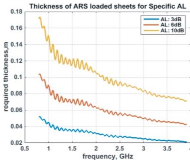
**Figure 4.** Thickness of ARS loaded panel for specific absorption loss.
