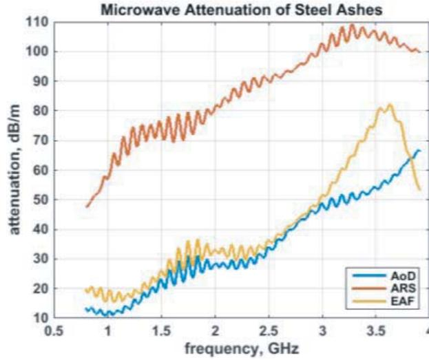
**Figure 3.** Microwave attenuation of steel ashes.
