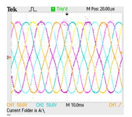
Figure 13. Oscillograms of the generator EMF.
