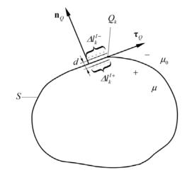
Figure 4. Section of a ferromagnetic sample along a segment  $\Delta l_k^I$ .
