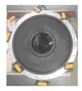
Figure 8. Axial flux machine stator.
