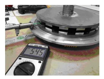
Figure 15. Measurement of the magnetic field in the non-magnetic gap of an electric machine.
