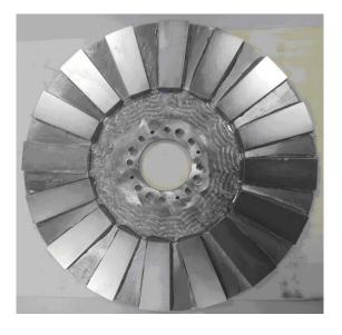
Figure 7. Axial flux machine rotor.
