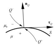
Figure 2. The boundary between the regions filled with ferromagnetic and air.
