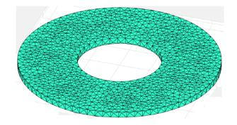
Figure 11. Triangulation of the disk surface.
