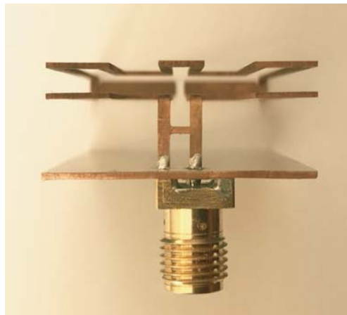
Figure 3. Photograph of the fabricated design D1 showing details of the SMA connector and feed.
