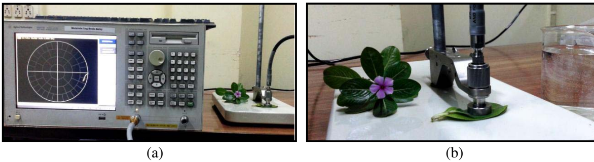
Figure 1. Dielectric properties measurement set up for Catharanthus roseus leaf samples with Agilent 85070E dielectric measurement kit and Vector Network Analyzer (VNA).
