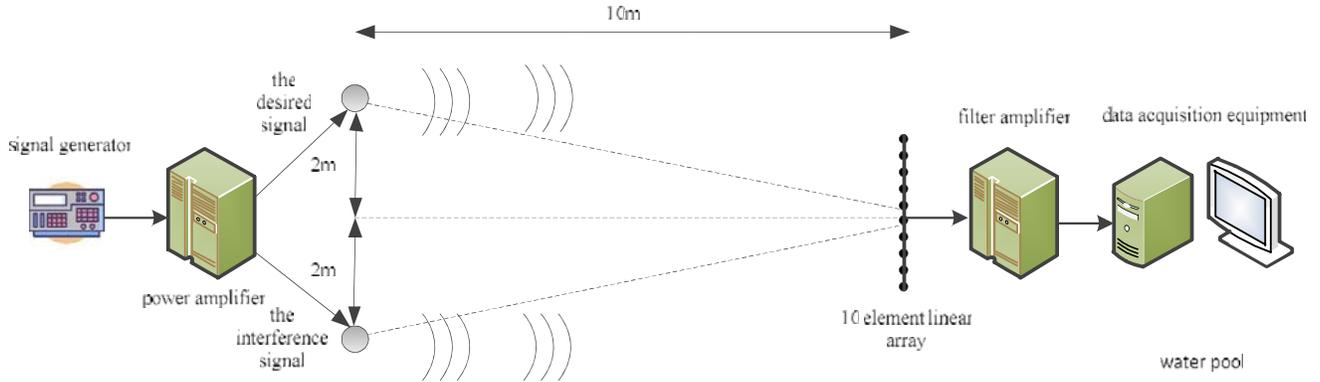
**Figure 6.** Layout of the water pool experiment.
