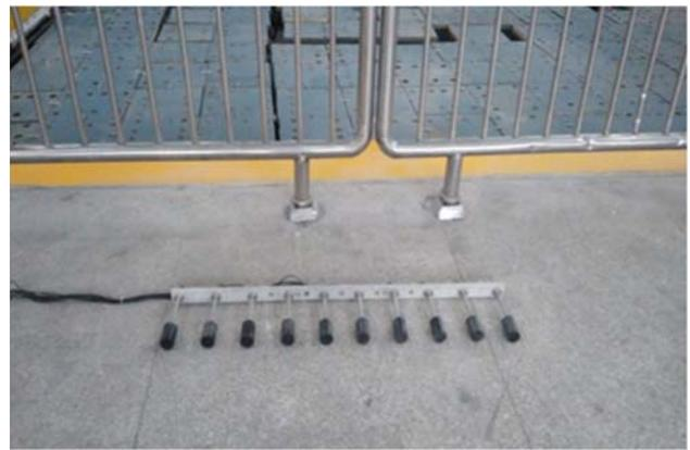
**Figure 8.** The 10-element linear array.
