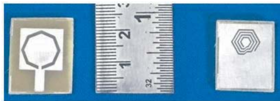
Figure 10. Photograph of the top view and bottom view of the proposed antenna.
