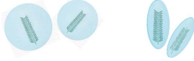
Figure 2. Two branches, each enclosed by a spherical surface (left figure) and a spheroidal surface (right figure), without overlap. The technique presented in this paper is suitable to treat any number of scatterers even though only two branches are shown in each sub figure.
