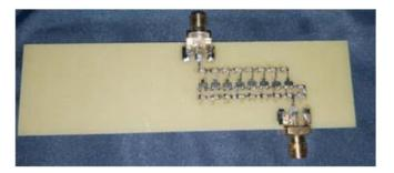
Figure 8. Fabricated rectifier circuit.
