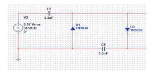
Figure 7. Single stage voltage doulber circuit.
