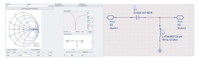
Figure 13. Impedance matching design for the 13 GHz RF to DC conversion circuit via ADS.
