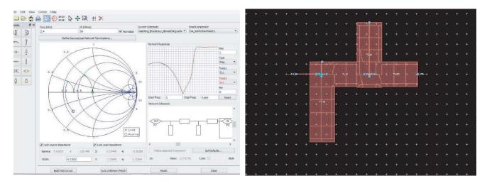
Figure 5. Impedance matching network design via ADS & transmission line calculator.
