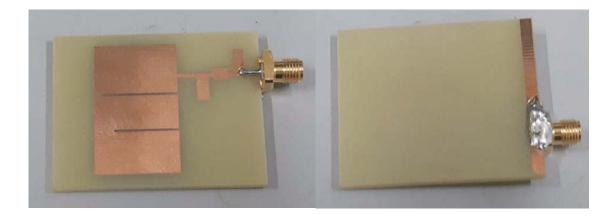
Figure 6. Fabricated E-shaped microstrip patch antenna together with the partial ground plane.
