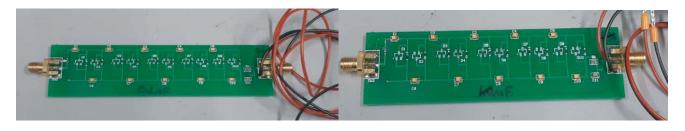
Figure 11. RF to DC conversion circuit fabricated to harvest the 70 MHz and 13 GHz signals.
