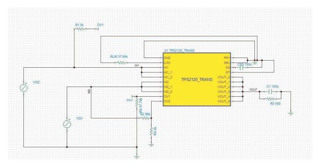
Figure 14. TPS2121 power management circuit.
