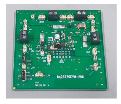
Figure 10. Fabricated BQ25570 power management circuit.
