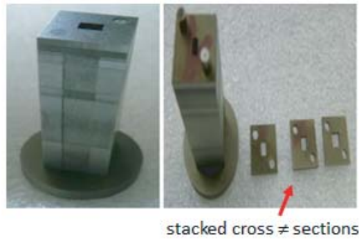
Figure 2. Prototype of the Design SHE antenna (radiating element and the RWG transition between the horn and a WR12 rectangular waveguide section). The dimensions of all the rectangular sections are given in Fig. 1.
