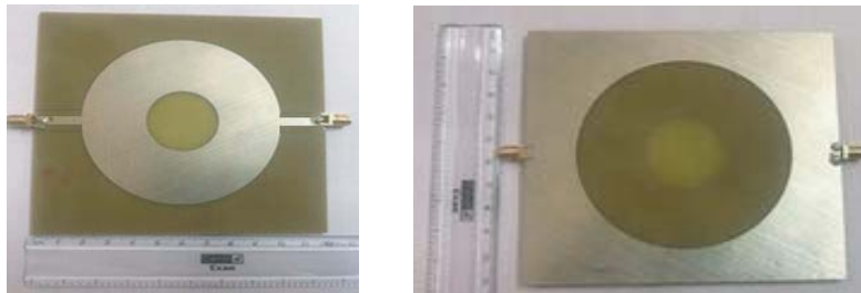
Figure 22. Top view and bottom view of fabricated proposed dual feed annular ring antenna.
