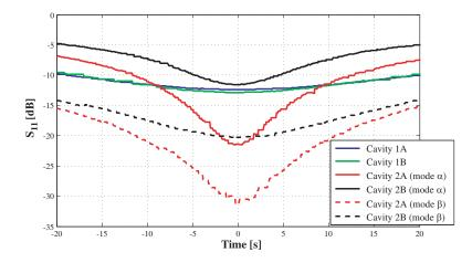
Figure 3. Thermal drift of the four cavities synchronized at their resonance. Incident power of 150 W.
