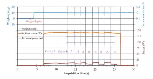
**Figure 4.** First experimental run chronogram gathering all the collected measurements. Small Shaker configuration (Cavities 1A & 1B), Fundamental mode. 20 mg calibration and then 200 W RF power at 2440 MHz.
