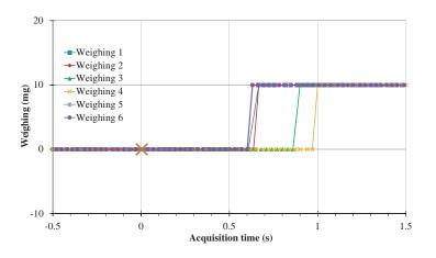
Figure 2. Calibration of the balance with the Big Shaker (Figure 1), mode  $\alpha$ . 6 measurements of a 20 mg weight video synchronized to the instant of contact (orange cross).
