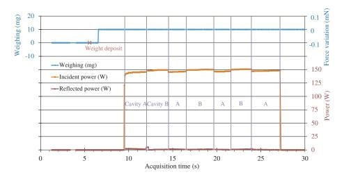
Figure 6. Third experimental run chronogram gathering all the collected measurements. Big Shaker configuration (Cavities 2A & 2B), Mode  $\beta$ . 20 mg calibration and then 200 W RF power at 2454.2 MHz.
