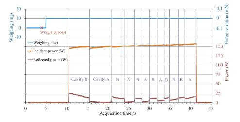
Figure 5. Second experimental run chronogram gathering all the collected measurements. Big Shaker configuration (Cavities 2A & 2B), Mode  $\alpha$ . 20 mg calibration and then 200 W RF power at 2442.2 MHz.
