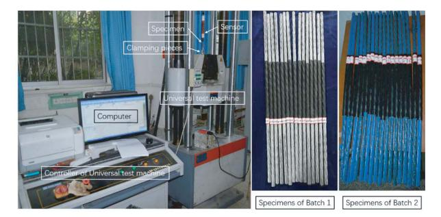
Figure 3. Experimental system and specimens.
