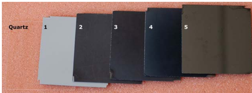
Figure 2. Photo of fabricated samples of resistive thin-film coatings with different oxygen content in the gas mixture in the process of magnetron sputtering on 60 \times 60 mm quartz slides. Samples numbering corresponds to Table 1.
