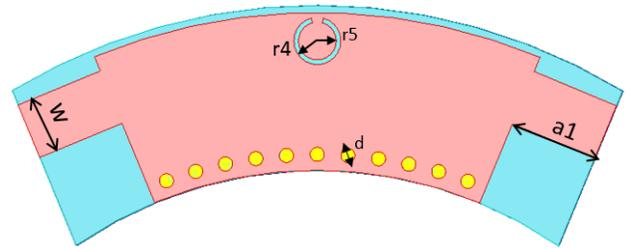
**Figure 3.** Configuration of the proposed UWB filter.
