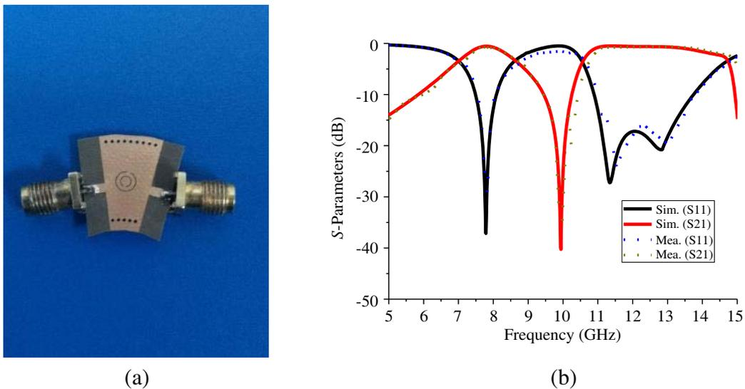
**Figure 7.** Photograph and comparison of the simulated and the measured results of the dual-band bandpass filter. (a) Photograph. (b)  $|S_{11}|$  and  $|S_{21}|$ .
