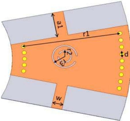
**Figure 2.** Configuration of the proposed dual-band filter.
