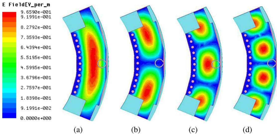
**Figure 5.** Simulated  $E$ -fields of the first four resonant modes in the proposed EMSIW cavity. (a) TM<sub>101</sub>, (b) TM<sub>102</sub>, (c) TM<sub>103</sub>, (d) TM<sub>104</sub>.
