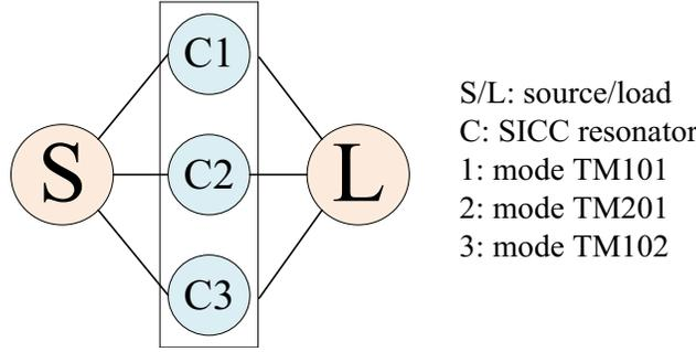
**Figure 6.** Coupling scheme of the dual-band filter.
