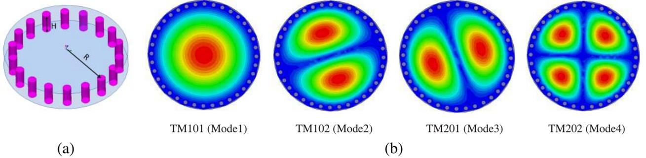
**Figure 1.** (a) Configuration of the SICC cavity. (b) Simulated  $E$ -fields of the first four resonant modes in the proposed cavity.
