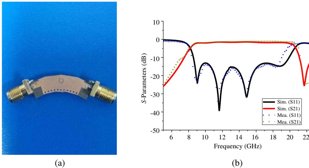
**Figure 8.** Photograph and comparison of the simulated and the measured results of the UWB bandpass filter. (a) Photograph. (b)  $|S_{11}|$  and  $|S_{21}|$ .
