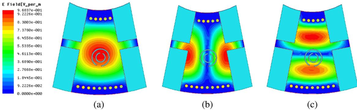
**Figure 4.** Simulated  $E$ -fields of the first three resonant modes in the proposed SMSIW cavity. (a) TM<sub>101</sub> (Mode1), (b) TM<sub>102</sub> (Mode2), (c) TM<sub>201</sub> (Mode3).
