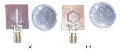
Figure 9. Prototype of FPEP antenna. (a) Radiating patch and (b) Ground plane.
