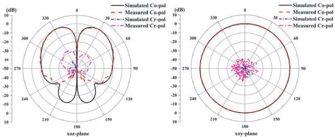
**Figure 11.** Measured and simulated normalized radiation patterns of the antenna at 3.40 GHz in *xoz*-plane and *xoy*-plane.
