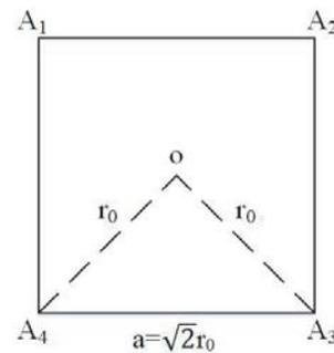
**Figure 2.** The mathematical derivation about the geometry length of a single rotating square patch.
