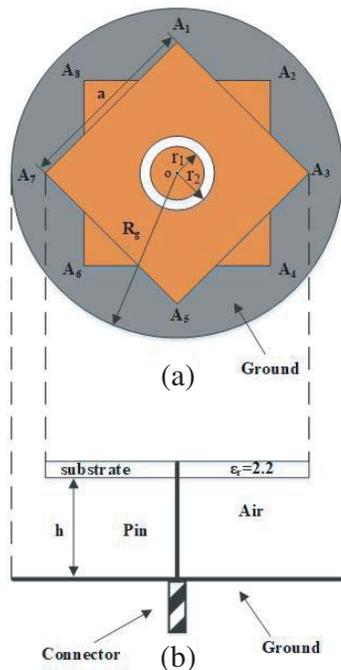
**Figure 1.** Geometry of the wideband omnidirectional microstrip patch antenna.
