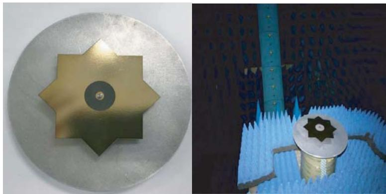
**Figure 10.** Photograph of the wideband omnidirectional microstrip patch antenna.
