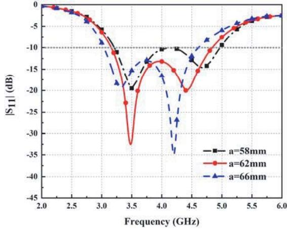
**Figure 5.** Simulated  $S_{11}$  curves at different values of  $a$ .
