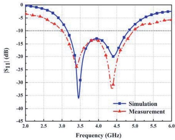
**Figure 8.** Simulated and measured return loss of the wideband omnidirectional microstrip patch antenna.
