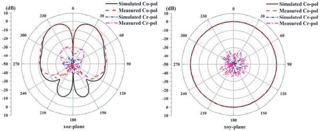
**Figure 12.** Measured and simulated normalized radiation patterns of the antenna at 3.80 GHz in  $xoz$ -plane and  $xoy$ -plane.
