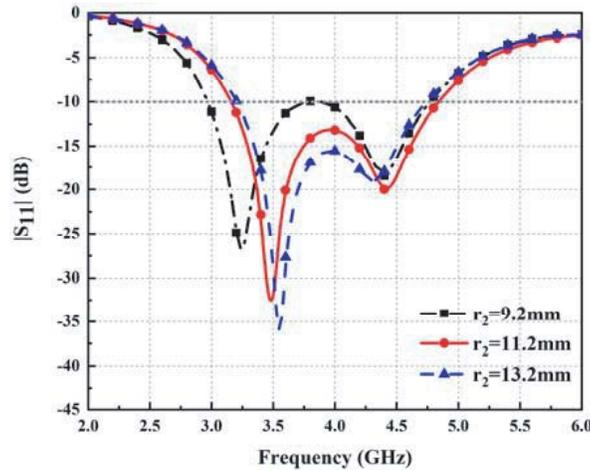
**Figure 7.** Simulated  $S_{11}$  curves at different values of  $r_2$ .
