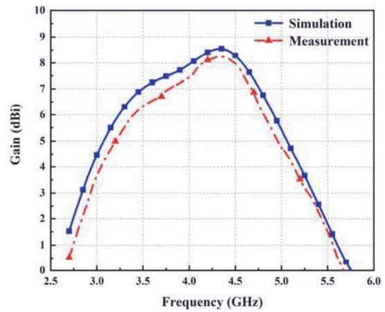
**Figure 9.** Simulated and measured gains of the wideband omnidirectional microstrip patch antenna.
