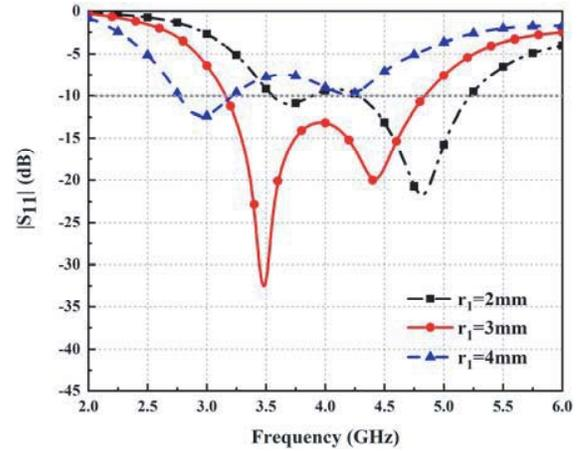
**Figure 6.** Simulated  $S_{11}$  curves at different values of  $r_1$ .
