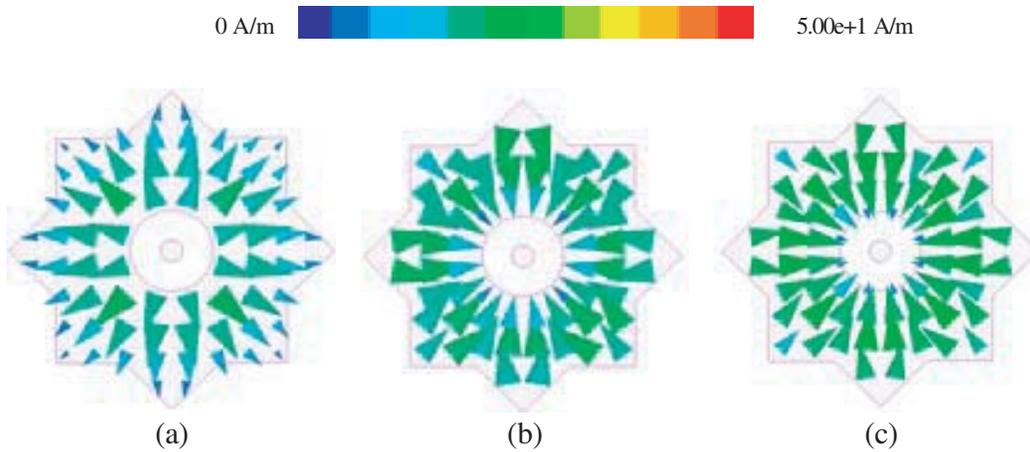
**Figure 4.** The current distribution of the proposed antenna: (a) 3.40 GHz, (b) 3.90 GHz and 4.40 GHz.
