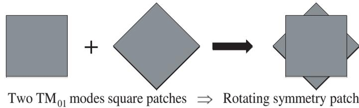
**Figure 3.** Geometry decomposition of the rotating square patches.
