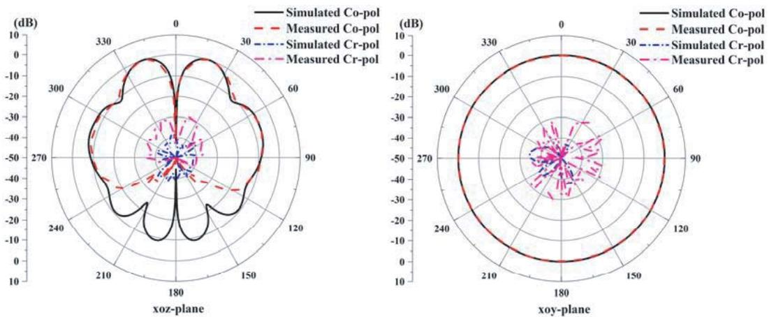
**Figure 14.** Measured and simulated normalized radiation patterns of the antenna at 4.80 GHz in  $xoz$ -plane and  $xoy$ -plane.
