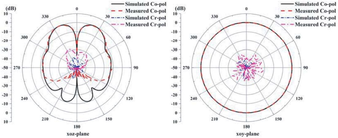
**Figure 13.** Measured and simulated normalized radiation patterns of the antenna at 4.20 GHz in  $xoz$ -plane and  $xoy$ -plane.
