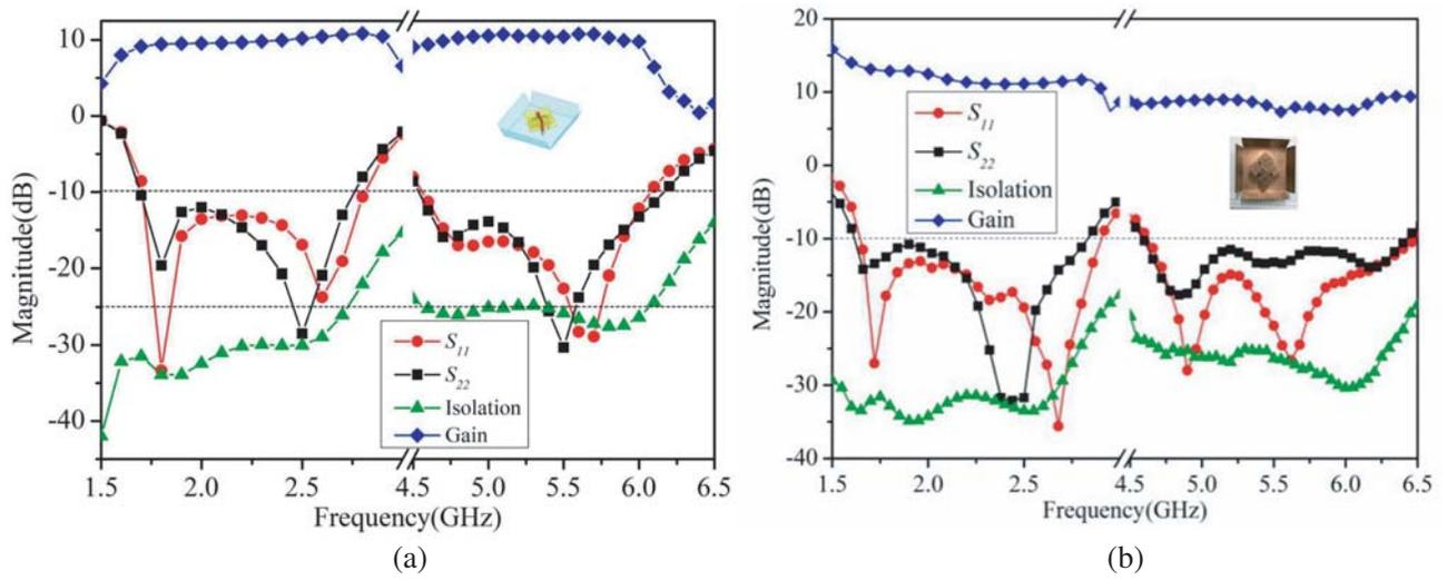
Figure 5. Simulated and measured results: (a) Simulated; (b) Measured.
