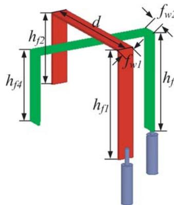
**Figure 2.** Geometry of the orthogonal  $\Gamma$ -shaped feeding line.
