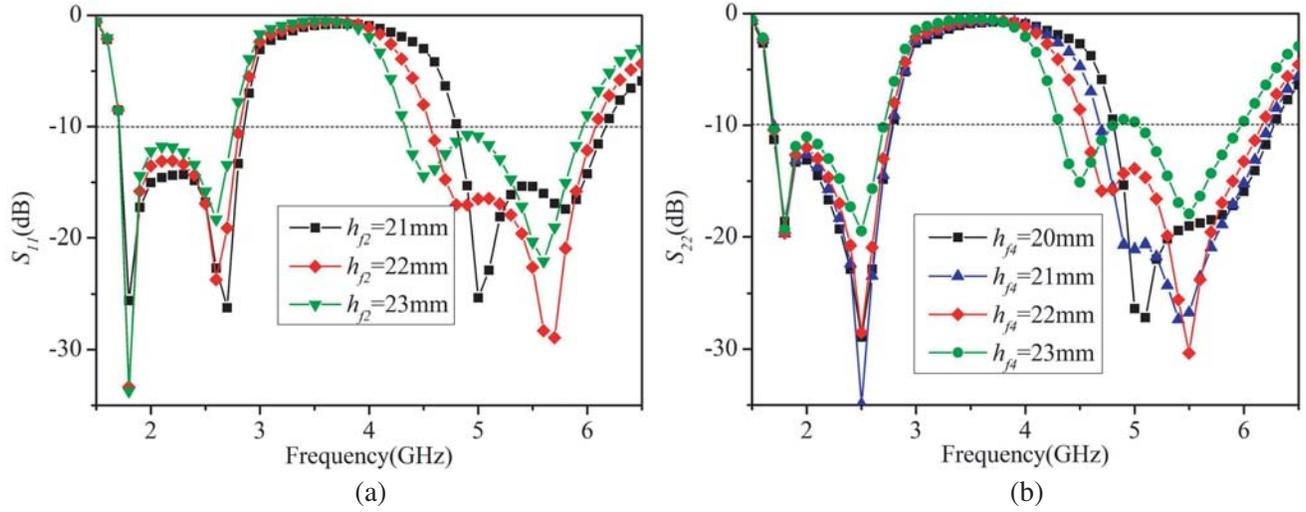
**Figure 9.** Effects of L-shaped feeding structure: (a) Effects of  $h_{f2}$  on  $S_{11}$ ; (b) Effects of  $h_{f4}$  on  $S_{22}$ .
