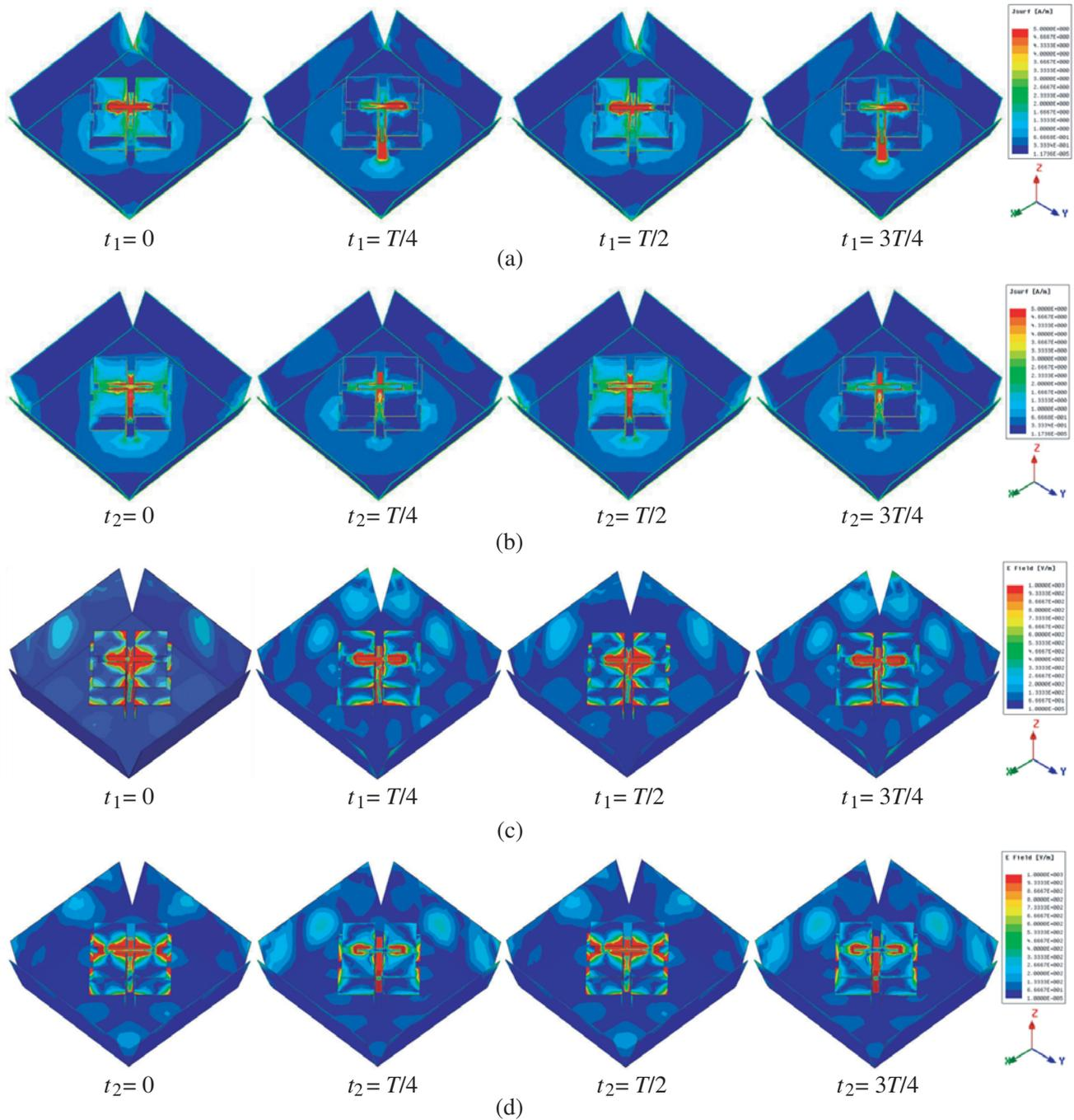
**Figure 3.** Current distributions of the dual-band dual-polarized antenna: 2.2 GHz (a) Port 1; (b) Port 2; 5.5 GHz (c) Port 1, (d) Port 2.
