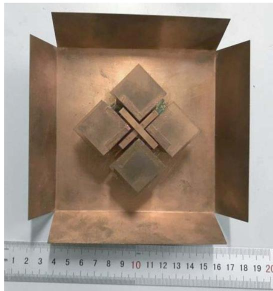
**Figure 4.** Prototype of the dual-band dual-polarized antenna.
