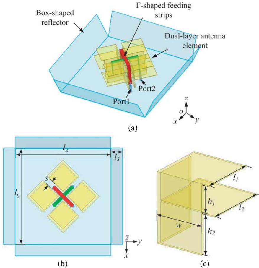
**Figure 1.** Perspective, top and side views of the dual-band dual-polarized antenna. (a) Perspective view; (b) Top view; (c) Side view.
