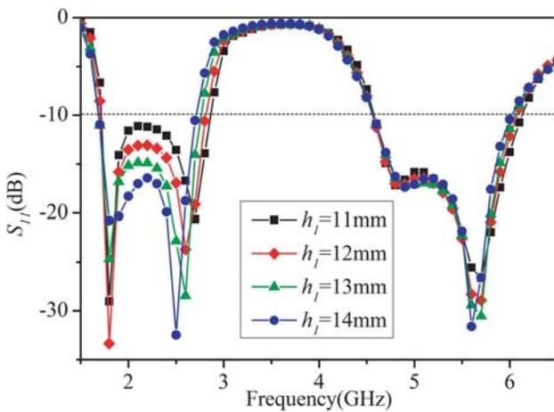
Figure 7. Effects of  $h_1$  on  $S_{11}$ .
