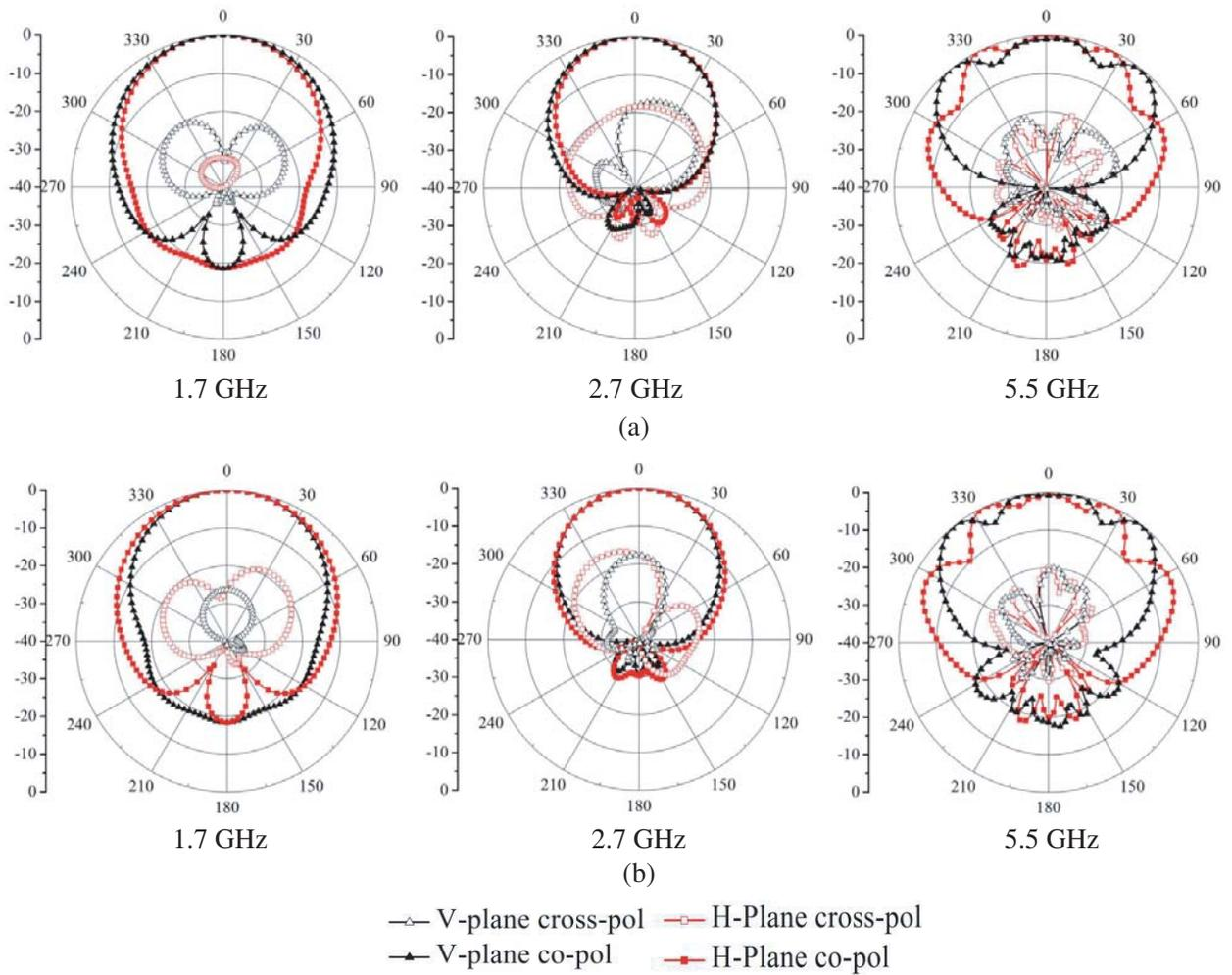
Figure 6. Radiation patterns of the antenna at frequencies of 2.2, 2.7 and 5.5 GHz. (a) Port 1; (b) Port 2.
