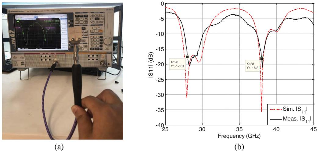
**Figure 11.** (a) Experimental setup for measuring the return loss of the dual-band antenna. (b) Measured frequency response of the return loss of the dual-band antenna compared with the simulation results.
