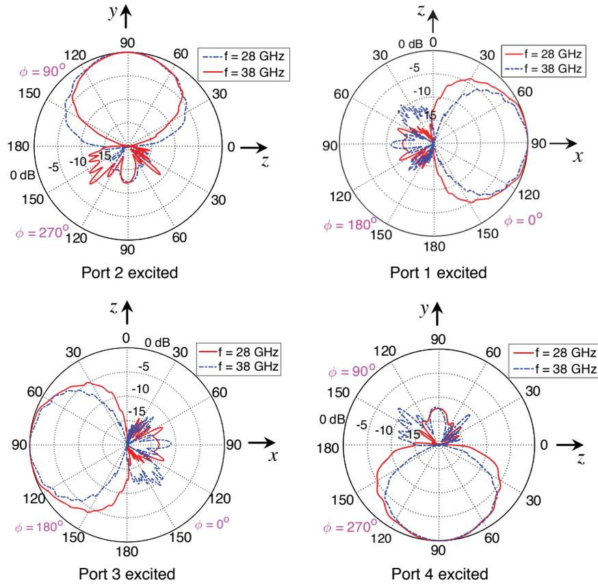
**Figure 8.** Radiation patterns in the plane normal to the antenna plane for the 4-port MIMO antenna using the proposed dual-band antenna at 28 and 38 GHz.
