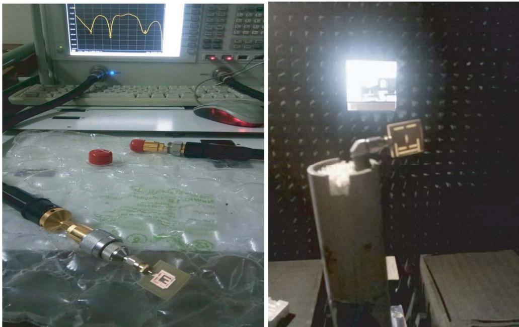
**Figure 8.** Measurement setup for the proposed antenna.
