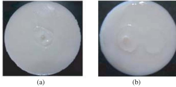
**Figure 3.** Fabrication of heterogeneous human breasts based on realistic T1-MRI images: (a) Type B, and (b) Type C models.
